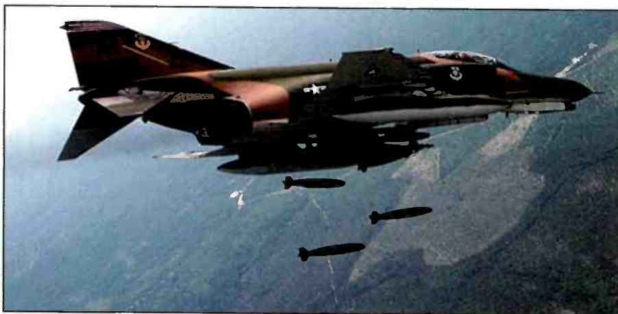
An F-4E from the 347th Tactical Fighter Wing dropping 500-pound Mark 82 bombs. (Public domain photo)
