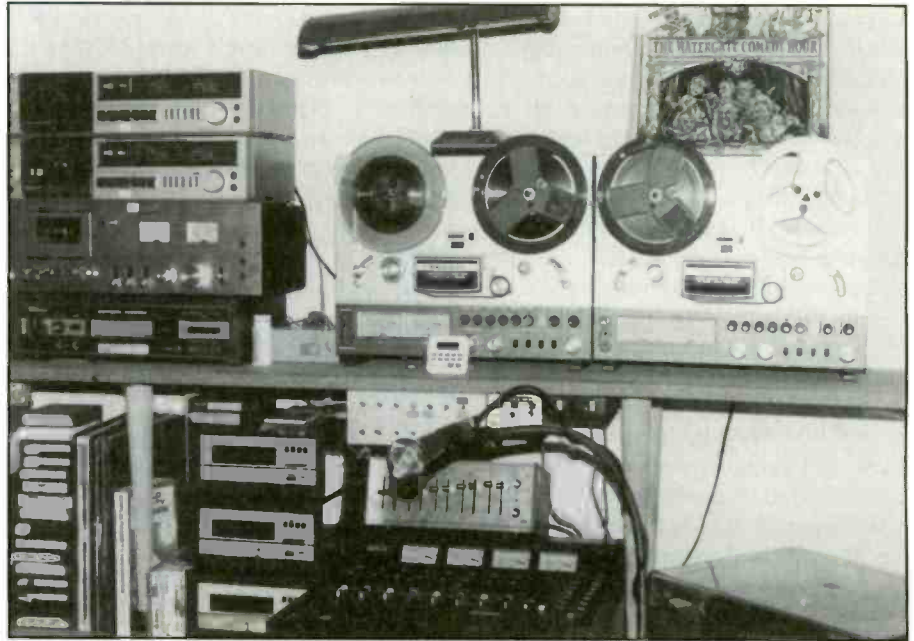
Photo C. A pair of open-reel tape decks (above right) in the studio of KKTO from the early 1980s. Also shown are cassette decks (to the upper left); carts and cart machines (lower left); microphone, equalizer, mixer (bottom center), and turntable (lower right).
