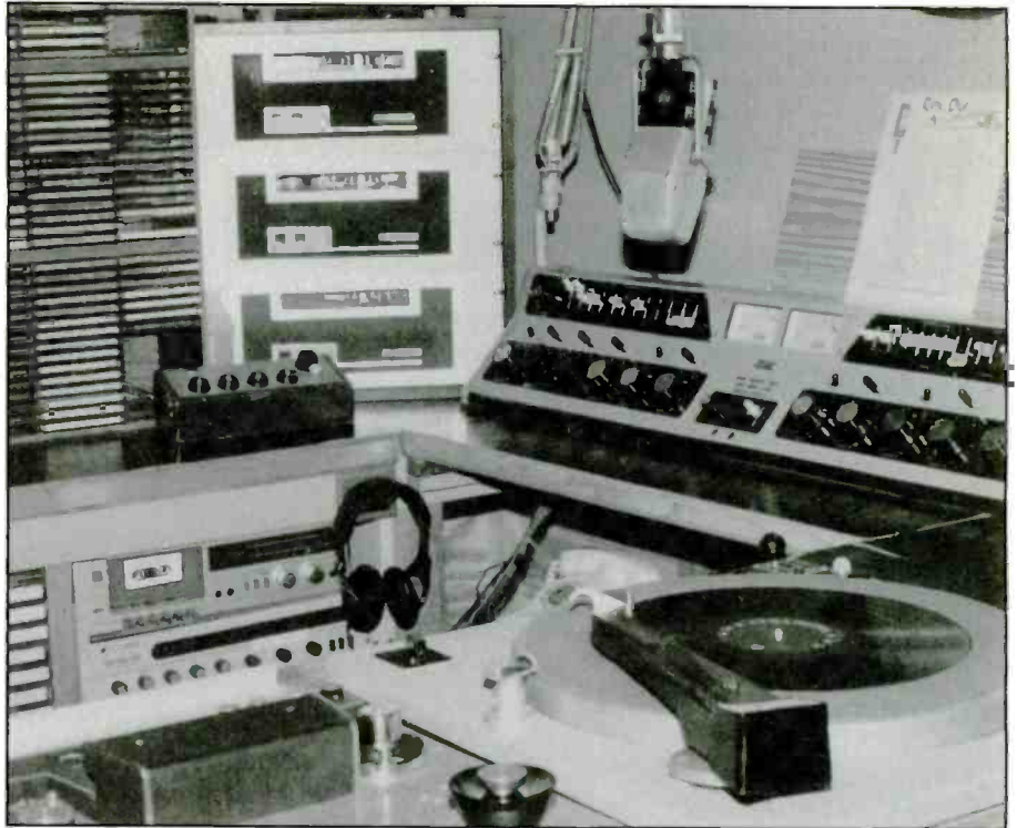
Photo B. The beautiful studio of Radio One, featuring classic broadcasting equipment. A stack of Gates cart machines can be seen at the upper center. To the right is an RCA ribbon microphone and an old broadcast console.
