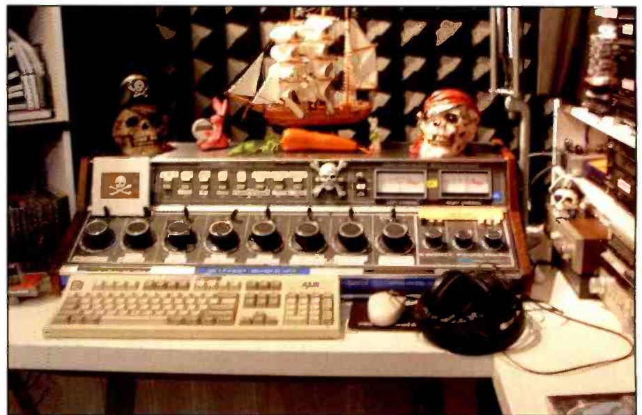
Photo D. The WBNY hybrid analog/digital studio, showing the professional broadcast console and computer keyboard in the center. To the right are stacks of cassette and CD decks.
