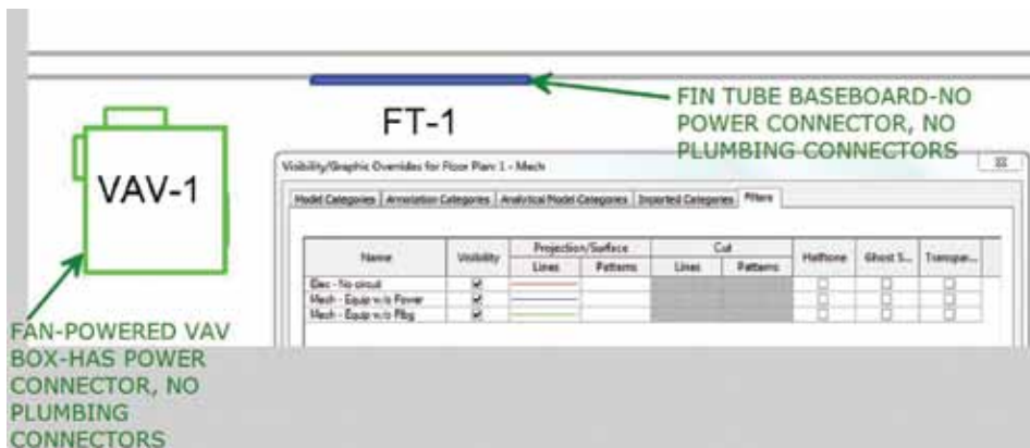
Figure 3: Moving the “without power” filter up in the list changes the priority of the filter that applies.
