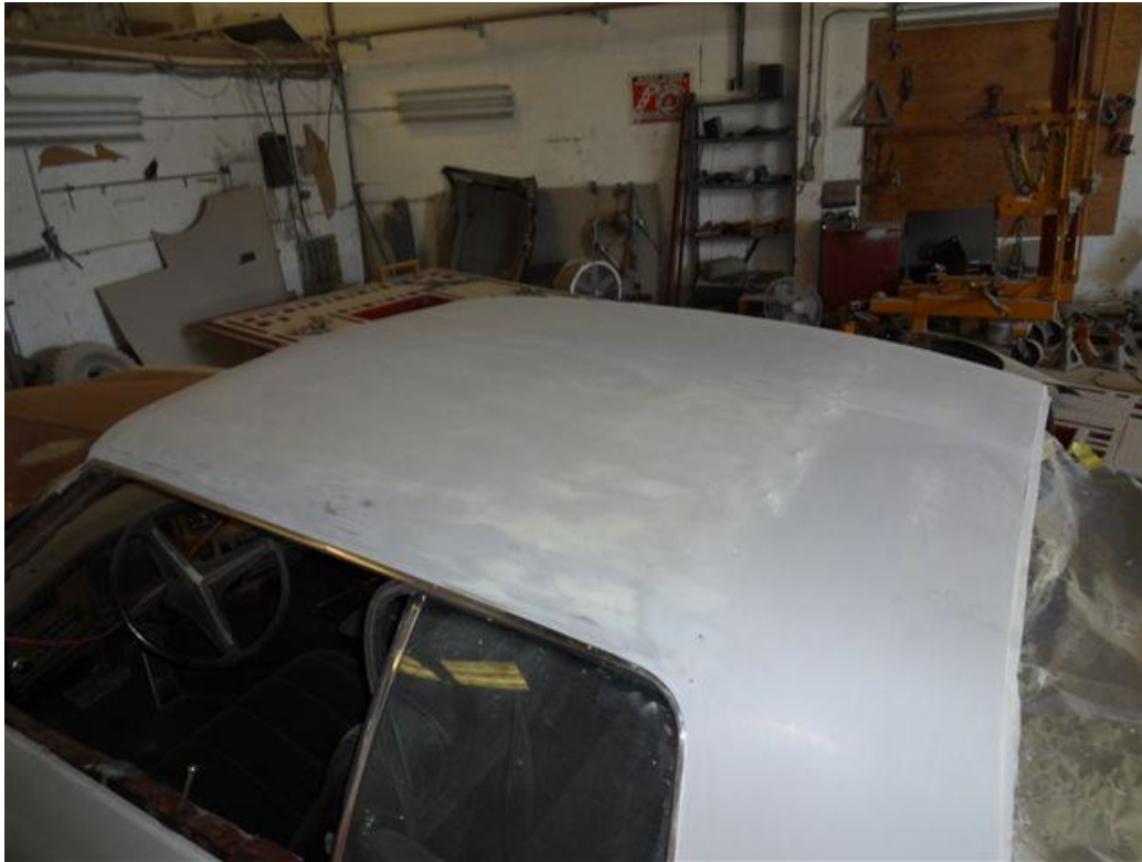
Roof of car. Vinyl and rust have been removed. New fiberglass has been applied.
