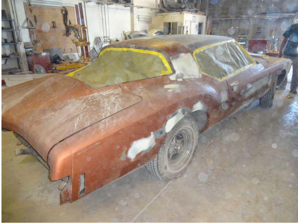
Coral all taped up, chrome removed and ready to start preparation for primer and paint
