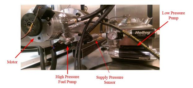
Figure 6: High Pressure Fuel Pump for 250bar
