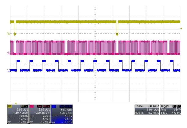
Figure 21: Pulse Signal for Solenoid Control Valve Synchronized with Crank Position Pulse
