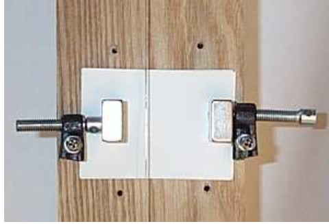
Figure 83: Lorentz' law type actuator (viewed from above)
