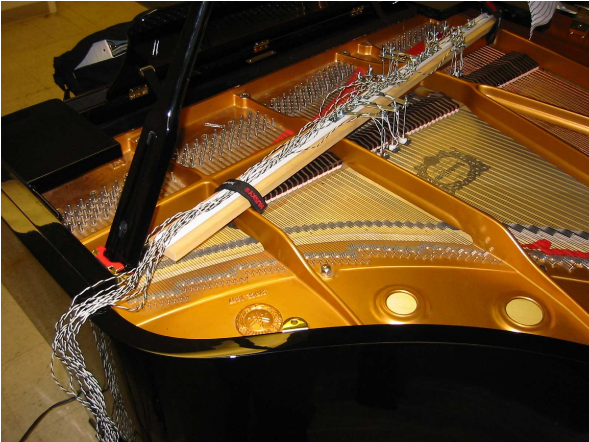
Figure 100: Electromagnetically prepared piano prototype
