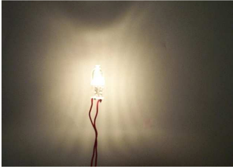
Figure 91: Nonuniform radiation pattern of a coiled halogen lamp
