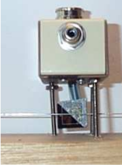
Figure 88: Photodiode type optical sensor in the laboratory (LED not shown)
