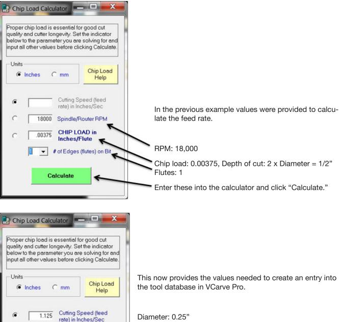
Diameter: 0.25" Pass depth: 0.5" Spindle speed: 18000 RPM Feed rate: 1.125 inches/sec
