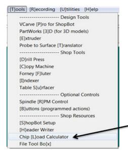
The "Chip Load Calculator" comes included in the ShopBot 3 software. It can be accessed by going to Tools > Chip Load Calculator (TL).
