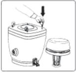
To attach the wheels, press the wheel posts into the four holes provided.
