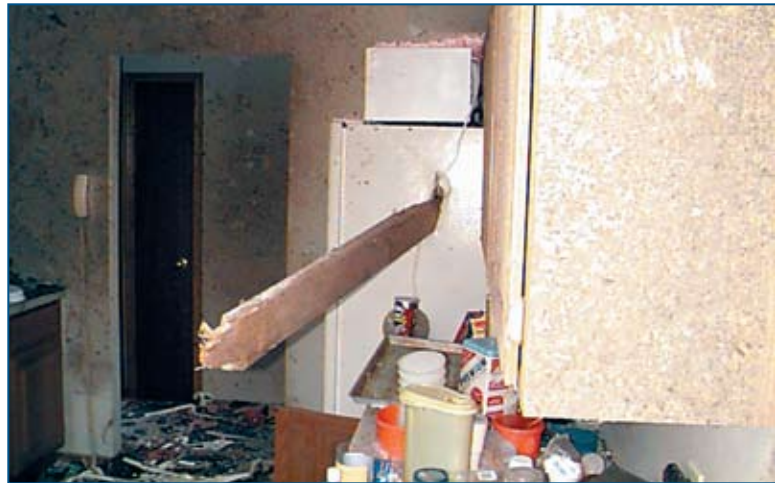
2" x 6" missile penetrating a refrigerator, midwest tornadoes of May 3, 1999
