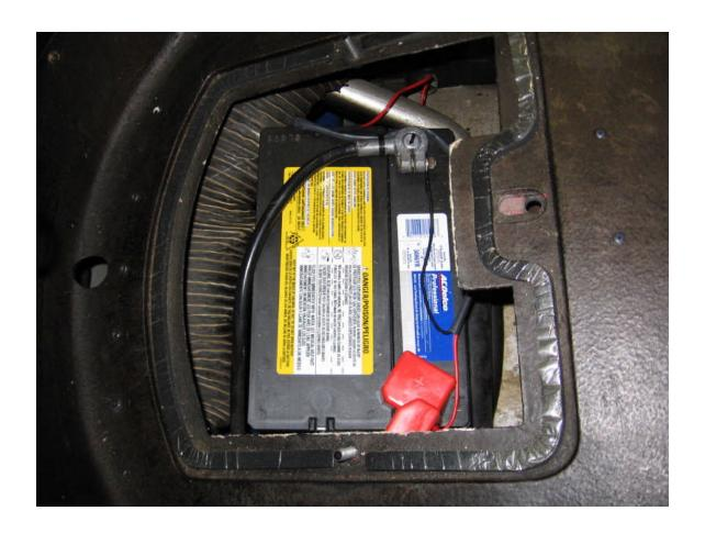
The harness then runs down and forward. Decide on length, clip the excess wire, and crimp each terminal. Each wire terminal then "clicks" into the white female connector. Check your charger to confirm, but on mine the black/ground wire went into the peaked end and the red/positive into the flat end:
