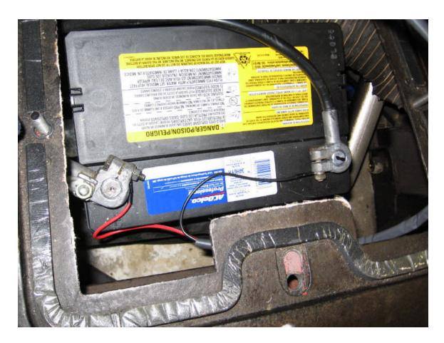
Route the red (positive) wire retrograde along the positive cable to clear the plastic cover. The cooling pipes run immediately behind the battery, so I zip-tied the harness directly to the negative cable terminal (if you are concerned regarding abrasion due to vibration, a short segment of vacuum hose slit lengthwise would provide good protection):
