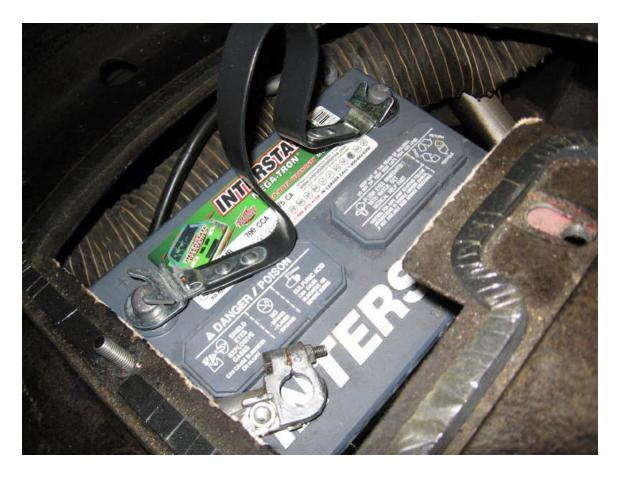
Clean up each terminal with terminal post tool. Drop the new battery into place and install hold-down clamp. Note opposite configuration of positive and negative terminals on the Delco battery compared with the previous Interstate (positive/negative remain on same side of car but battery is in opposite orientation):
