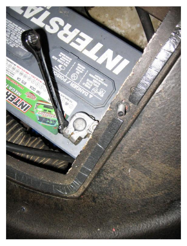
The hold-down clamp is located in the front center. Using a 13mm deep socket on a long extension, loosen and remove the clamp plate, nut, and lockwasher:
