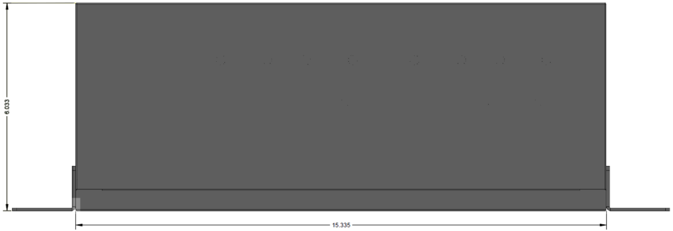
Dimensions with brackets attached for rack mounting (front view)
