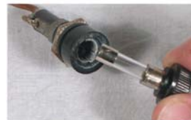
Panel fuse holder with glass fuse
