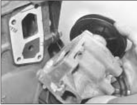
9.21 Fitting coolant pump (1116 cc engine)
