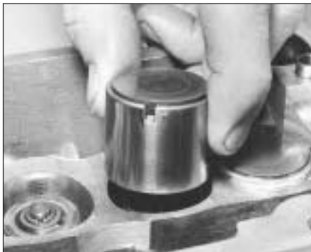
5B.25B Removing a cam follower (tappet) with shim
