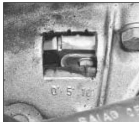
10.2B Flywheel timing marks (1372 cc ie engine)
