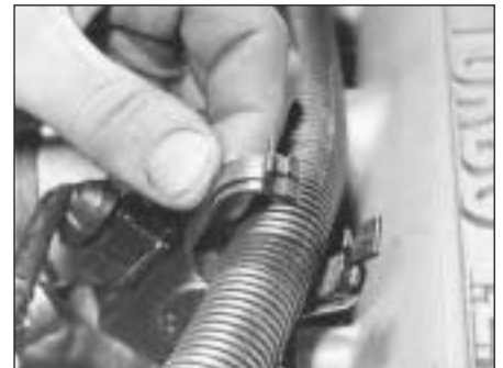
9C.77 Wiring loom clip and bracket
