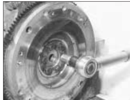
5D.14 Tightening a flywheel bolt
