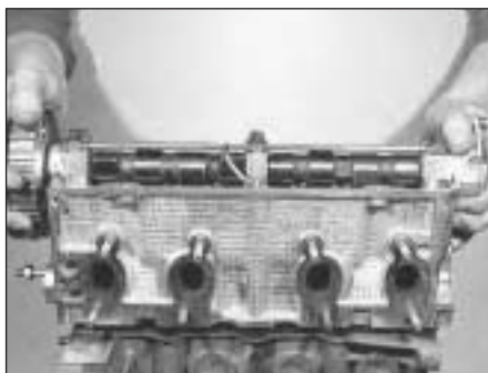
5B.51 Fitting the cylinder head
