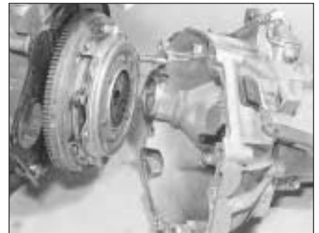
44.1 Offering transmission to engine
