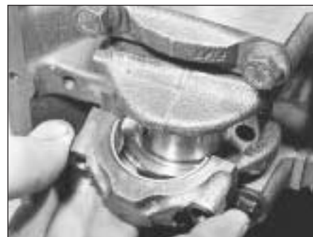
5B.98 Fitting a big-end bearing cap
