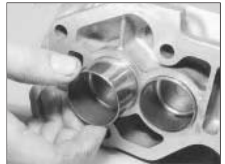
39.10 Cam followers fitted to camshaft carrier
