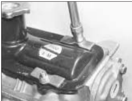
42.26 Tightening a camshaft carrier cover nut
