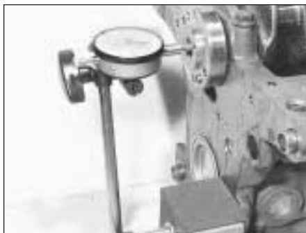
5D.8 Checking crankshaft endfloat using a dial gauge
