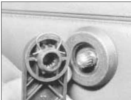
11.4 Window regulator handle removed
