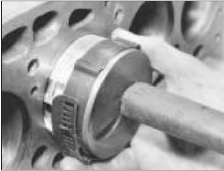
32.14 Fitting piston into cylinder bore
