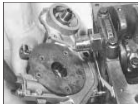
5B.78 Fitting the oil pump
