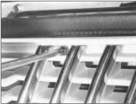
17.19A Extracting a radiator grille screw
