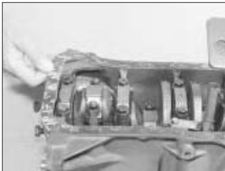
30.5 Locating the sump pan gasket
