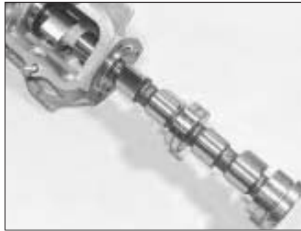
27.13B Withdrawing camshaft from carrier
