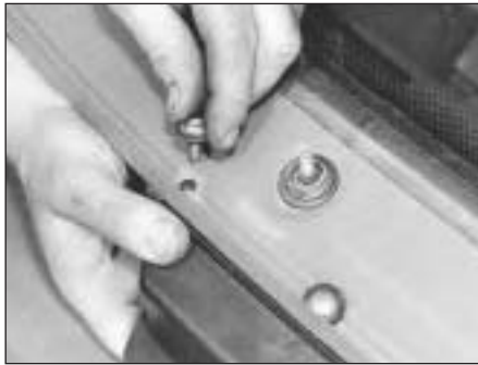
15.98A Remove the wiper motor retaining screws . . .
