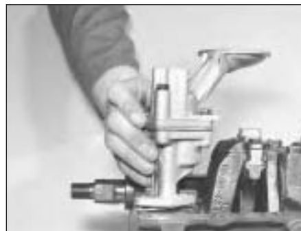
10.4 Fitting the oil pump
