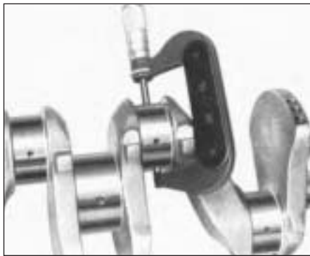
Fig. 1.25 Checking a crankpin (Sec 18)
