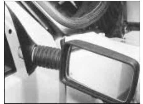
24.4 Withdrawing exterior mirror and trim plate
