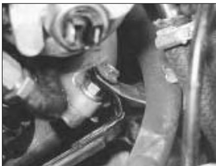
9C.72 Double nuts at the end of the inlet manifold
