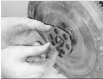
7B.158A Locate the flywheel, washer plate and bolts . . .
