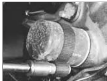
7A.12B Engine oil filter removal using a strap wrench - 1372 cc engine
