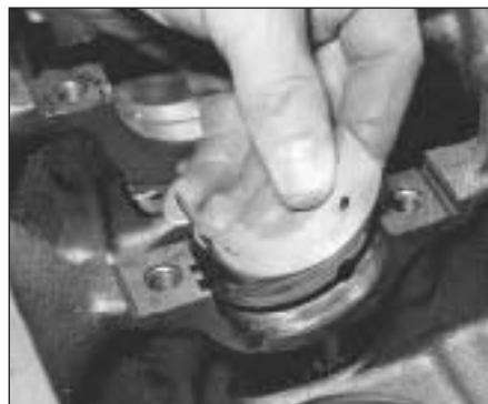
7D.6A No. 3 main bearing shell is plain . . .
