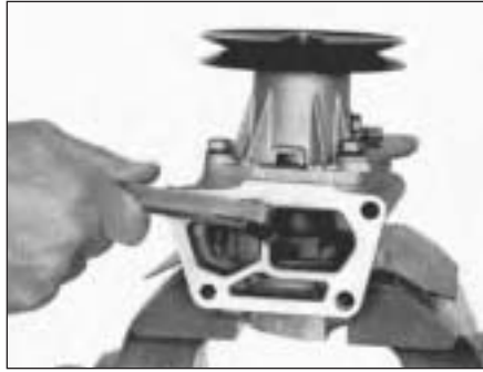
Fig. 2.6 Checking impeller clearance (Sec 9)
