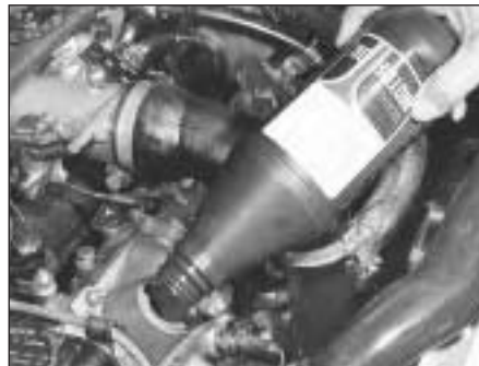
6C.27 Filling the engine with oil
