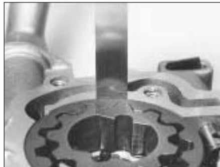
5B.74A Checking the oil pump gear-to-housing clearance
