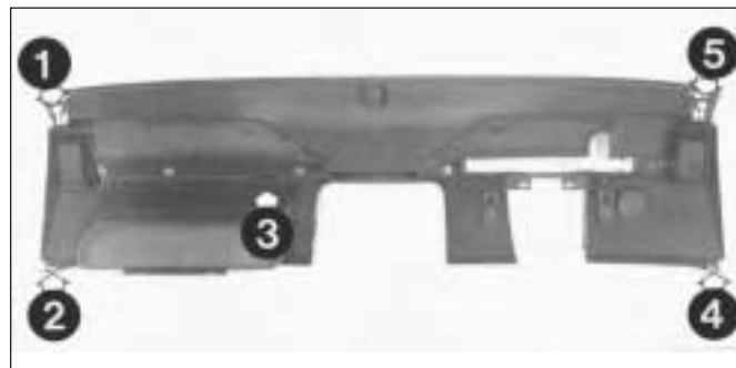
Fig. 12.20 Rear view of fascia panel showing fixing screw locations (Sec 22)
