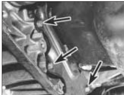
12B.33 Lower cover plate and retaining bolts (arrowed)
