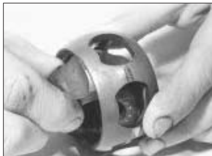
13.19B Separating inner and outer cage members
