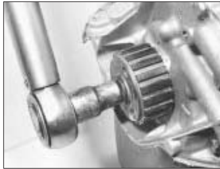
5D.16B Tightening the crankshaft sprocket bolt
