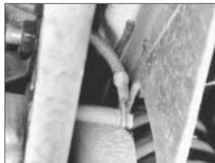
7C.33 Disconnect the transmission earth strap
