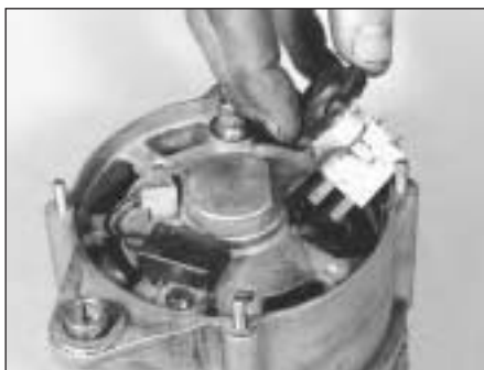
15.16B Removing the alternator brush holder
