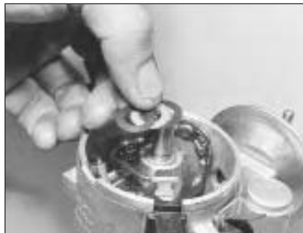
2.22B Washers above contact breaker
