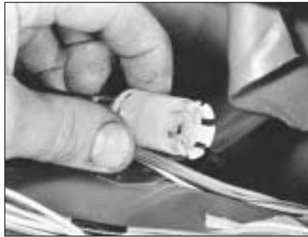
15.59B . . . and disconnect the speedometer cable
