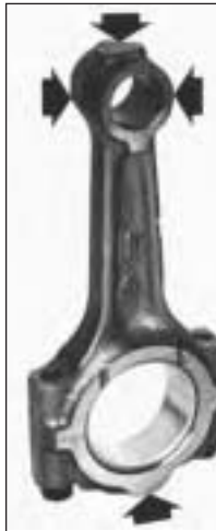
Fig. 13.7 Metal removing areas (arrowed) on connecting rod - 999 and 1108 cc engine (Sec 5C)
