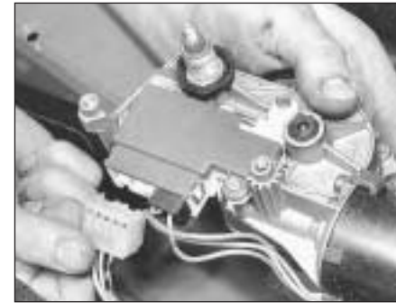
15.98C . . . and detach the wiring connector
