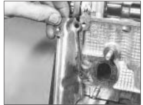
5D.20 Fitting the timing belt rear cover
