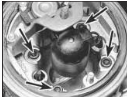
9D.44 Injector unit retaining screws (arrowed)
