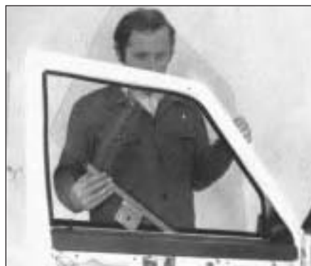
Fig. 12.8 Removing door glass (Sec 12)
