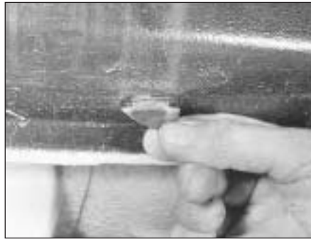
2.4B Sill drain with non-return valve
