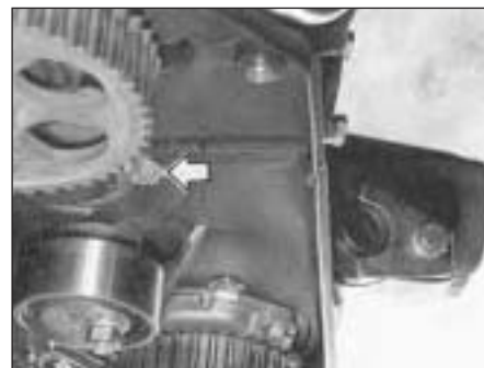
Fig. 13.18 Timing belt rear cover bolt (arrowed) - 1372 cc ie and Turbo ie engines (Sec 7B)
