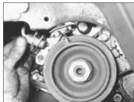
6B.19A Removing the TDC sensor
