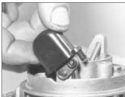
9B.23A Choke linkage cover removal from the Weber 32 TLF carburettor
