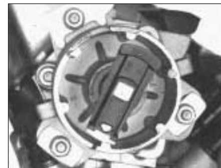
Fig. 13.78 Rotor aligned with distributor body rim mark - Microplex ignition system (Sec 10)
