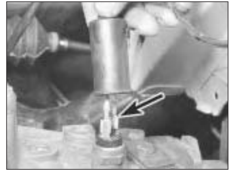
44.22A Reversing lamp switch on transmission
