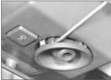
15.80A Prising free the roof-mounted spotlamp
