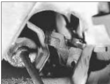
15.13 Driveshaft bracket swivelled downwards
