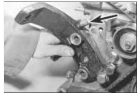
42.24C Engine mounting bracket with belt tensioner plunger (arrowed)
