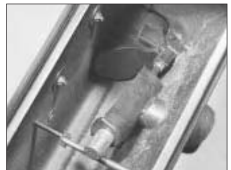
9A.7 Air cleaner thermostatic flap opener on the 999 cc model
