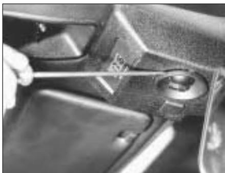
15.82 Roof-mounted clock retaining screw removal
