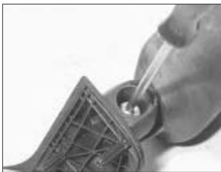
17.8 Extracting the mirror balljoint screw
