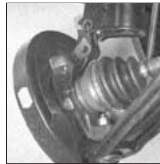
Fig. 1.18 Hub carrier detached from strut clamp (Sec 13)
