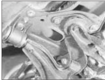
6.3 Track control arm inboard fixing
