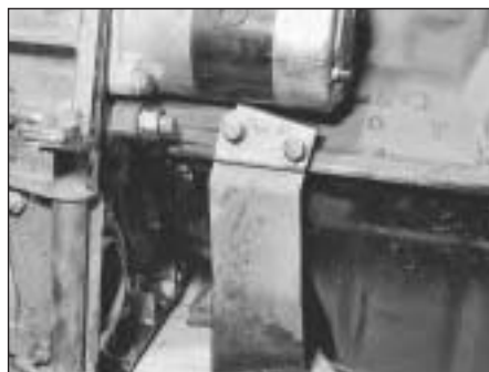
5C.60B Exhaust pipe support bracket attached to crankcase
