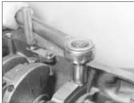
42.4B Tightening a main bearing cap bolt
