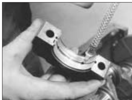
7D.9 . . . and lubricate the shells
