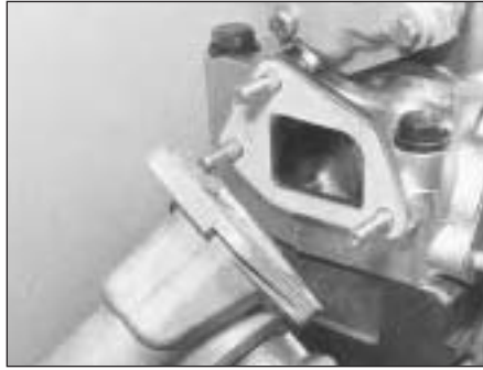
4.4 Fitting thermostat housing (1116 cc engine)
