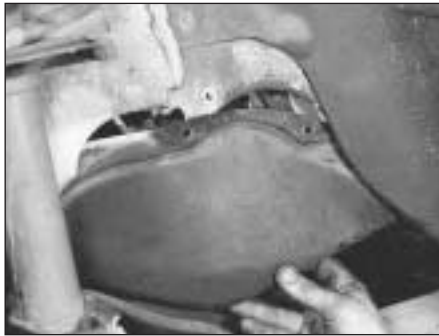
15.8 Remove the wheel arch lower guard panel for access to the alternator
