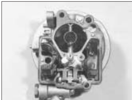
9B.23C Underside view of the cover on the Weber 32 TLF carburettor
