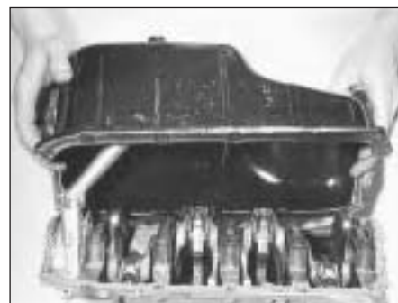
5C.60A Removing the sump pan
