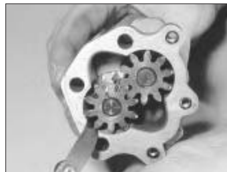
7B.176 Check gear-to-body clearance
