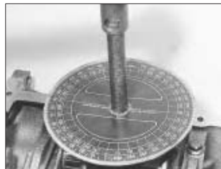
5D.7B Angle-tightening a main bearing cap bolt
