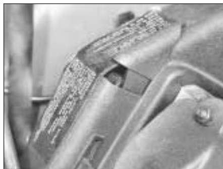
7B.29 Slide back inspection cover in the timing case
