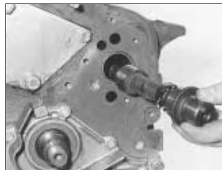
7C.54 Inserting the auxiliary shaft into the cylinder block (rear timing belt cover removed)
