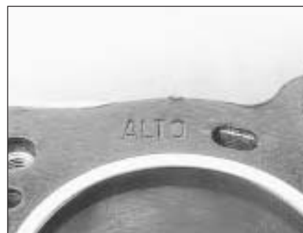
5B.50B Cylinder head gasket top surface marking
