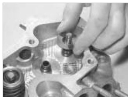
7B.130E Refit the flat washer . . .
