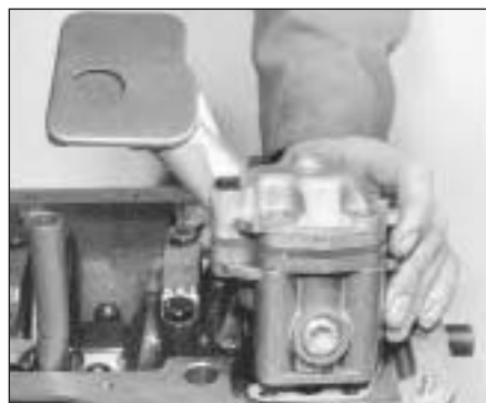
42.13 Locating oil pump and gasket
