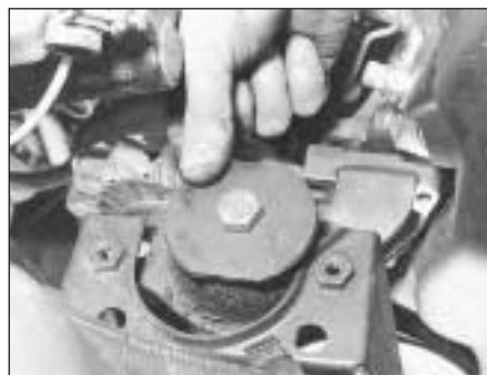
5C.31A Right-hand engine mounting disconnected
