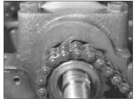
6.13C Self-tensioning links on inside of chain
