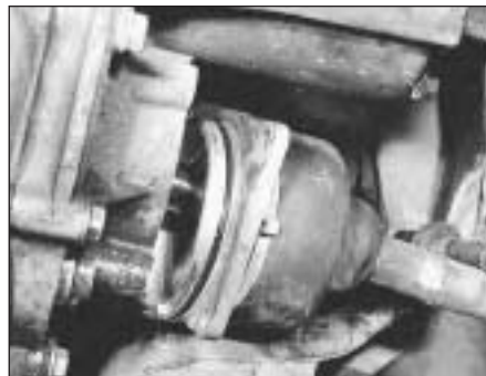
5C.25B Driveshaft joint gaiter withdrawn
