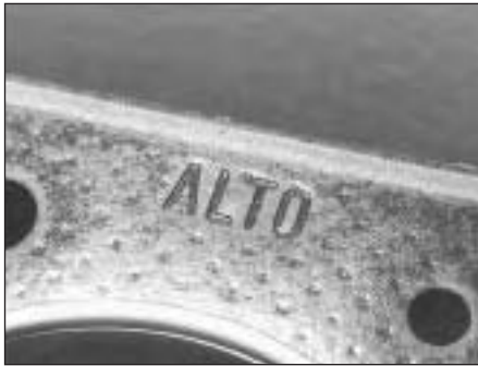
29.21A Cylinder head gasket top face marking
