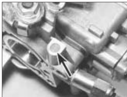
9B.8 Weber 32 TLF 4/250 carburettor mixture screw location under tamperproof plug (arrowed)
