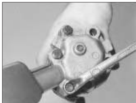
7B.171 Undo the oil pump cover bolts
