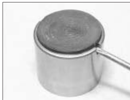
26.2 Removing a shim from a cam follower
