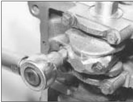
5B.99 Tightening a big-end cap bolt
