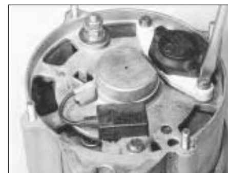
15.16A Extracting the alternator brush holder screw
