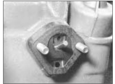
3.6B Fuel pump spacer and pushrod
