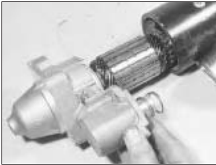
9.8 Starter motor dismantled
