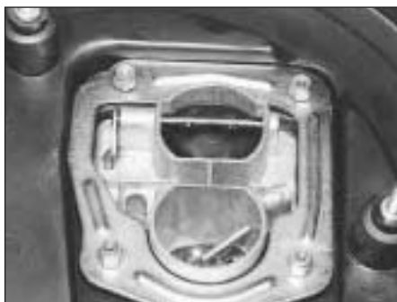
9A.9A Circular type air cleaner fixing nuts
