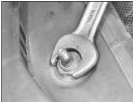
15.95 Unscrewing the wiper pivot nut
