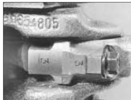
5B.88 Connecting rod and cap numbers
