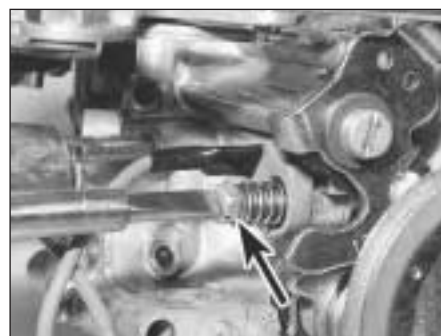
9B.36A Showing idle speed screw (arrowed) and . . .
