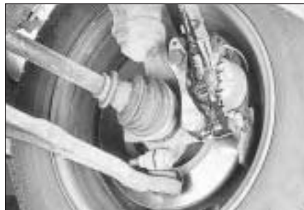
A leak occurring at a wheel is almost certainly brake fluid.
