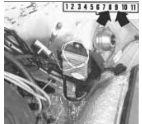
Fig. 4.13 Test lamp connected between terminals 8 and 9 of control unit multi-plug (Sec 10)
