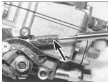
9B.6 Weber 32 TLF 4/250 carburettor idle speed screw (arrowed)
