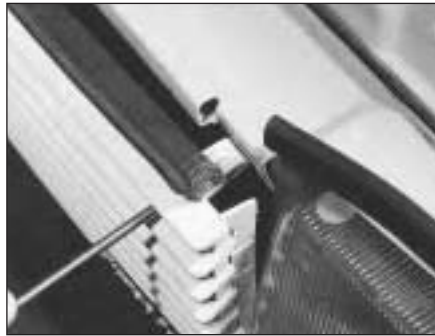
17.19B Prising down a radiator grille clip
