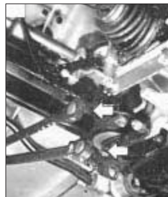
Fig. 13.25 Gear engagement and selector lever balljoints (arrowed) on the 1372 cc ie and Turbo ie engines (Sec 7C)
