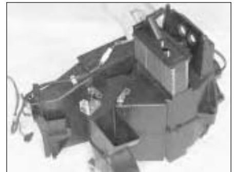
Fig. 2.10 Withdrawing heater matrix (Sec 13)
