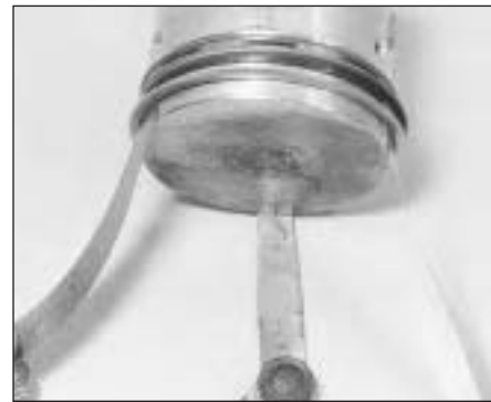
18.20 Using feeler blades to fit piston rings
