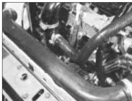
9C.55D Air cleaner metal duct over radiator
