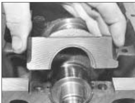
5D.6 Fitting a main bearing cap
