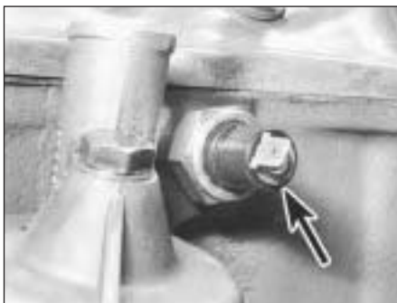
44.26A Oil pressure warning switch
