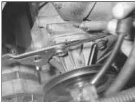
8C.40 Coolant pump/alternator bracket bolt removal
