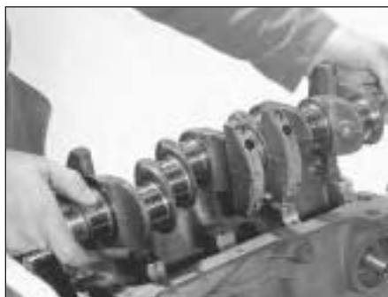
7D.10 Lower the crankshaft into position
