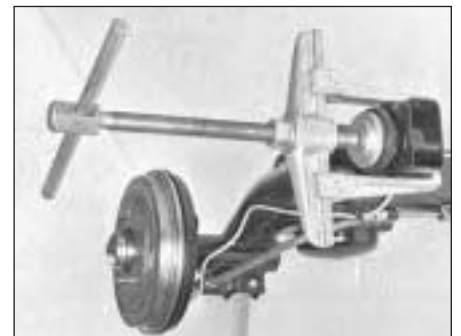
Fig. 11.10 Method of renewing trailing arm bush (Sec 10)
