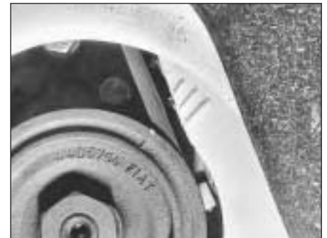
4.4 Ignition timing marks on belt cover
