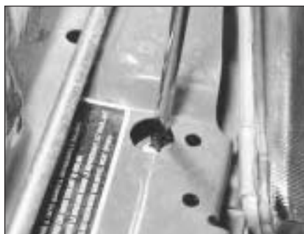
15.31A Headlamp horizontal beam alignment adjuster screw on a 1372 cc ie model
