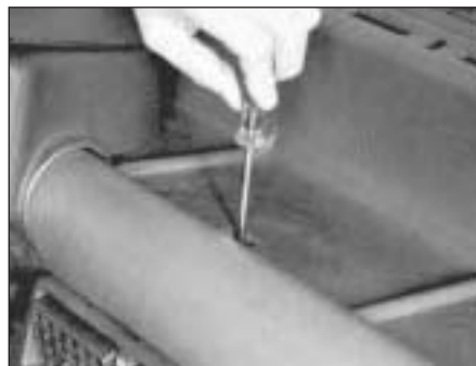
Fig. 2.8 Extracting heater upper fixing screw (Sec 12)
