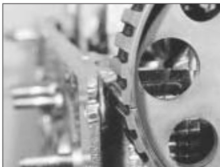
5B.8A Camshaft sprocket timing mark and cylinder head timing mark in alignment
