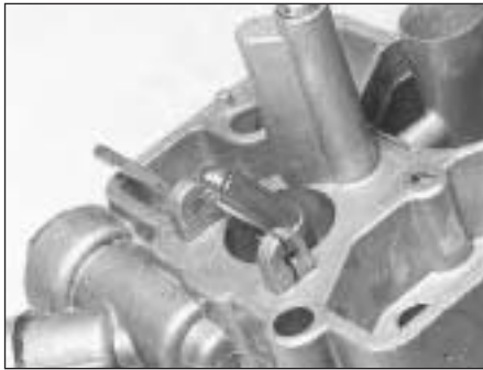
9B.26C Fuel inlet valve body and washer removal from the Weber 32 TLF carburettor
