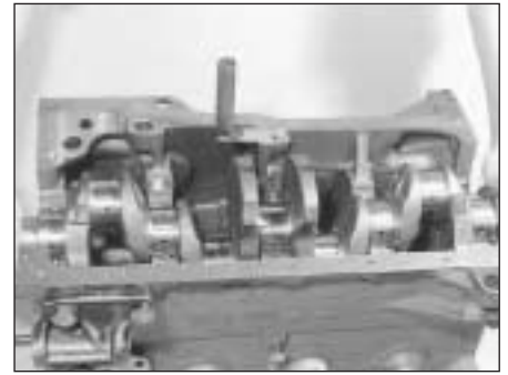
42.3 Lowering crankshaft into position
