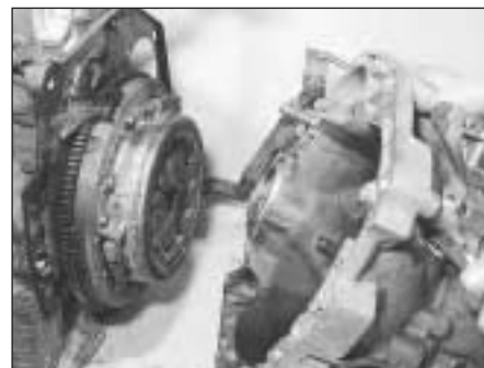
5C.39 Separating the engine and transmission
