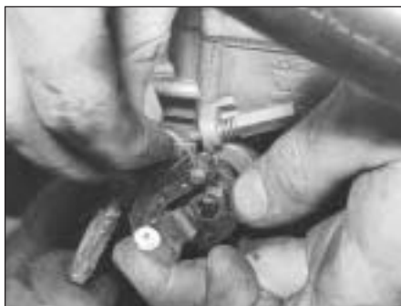
5B.32 Disconnecting the throttle cable
