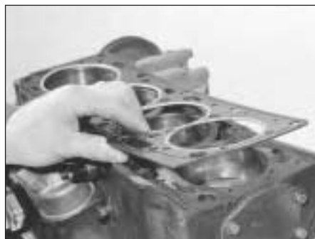
7B.119 Locating a new cylinder head gasket on the cylinder block (engine shown on dismantling stand)
