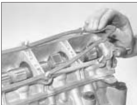
7B.89A Locate a new gasket on the camshaft housing . . .
