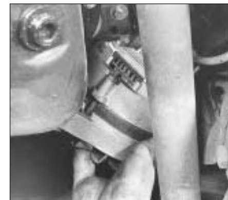
15.4 Removing the alternator from the 999 cc engine
