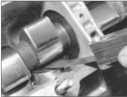
7B.10 Measuring a valve clearance (No 2 valve shown)
