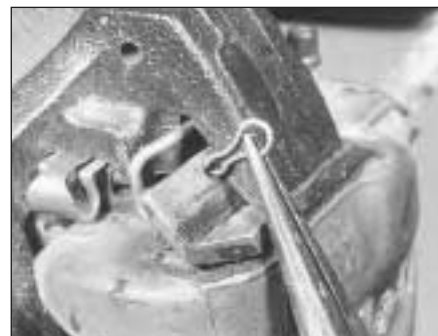
3.2A Removing a disc pad locking block clip
