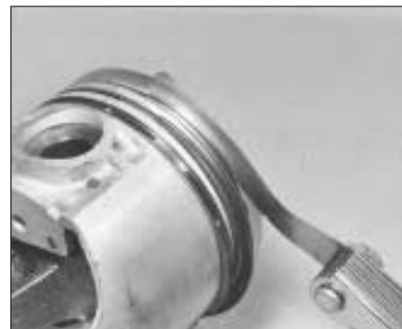
18.24A Checking piston ring groove clearance
