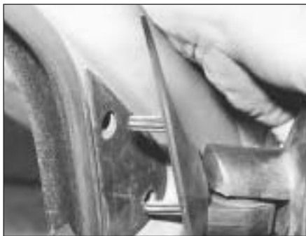
17.7B Withdrawing the exterior mirror
