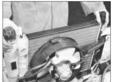
7.4B Removing radiator/fan assembly
