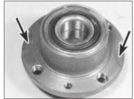
4.11 Rear hub showing cut-outs on rear face for shoe self-adjuster bosses
