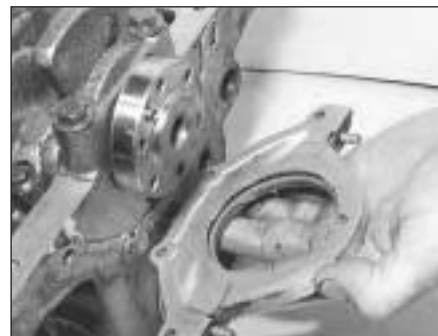
5D.9 Fitting crankshaft rear oil seal retainer
