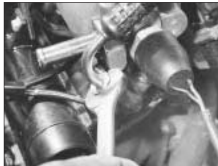
9C.75 Disconnecting the fuel delivery hose union
