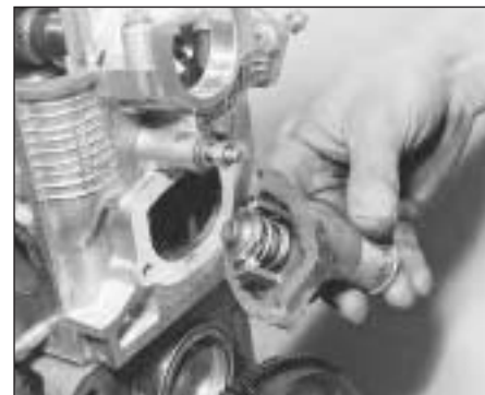
8A.9 Fitting the thermostat housing. Note the new gasket
