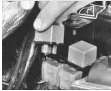
9D.27 Fuel pump relay removal
