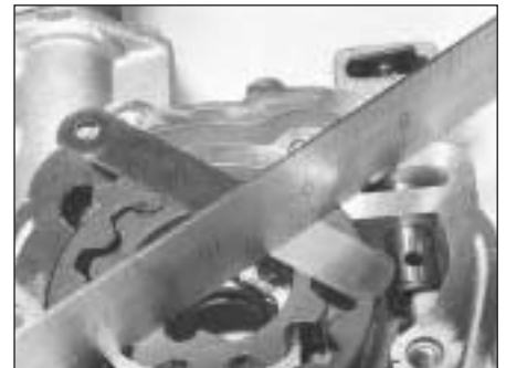
5B.74B Checking the oil pump gear endfloat
