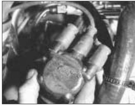
10.38 Removing the distributor cap
