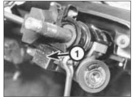
11.4 Unscrewing steering column switch clamp nut
