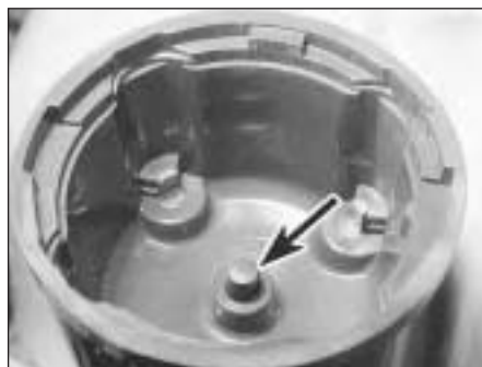
2.16 Interior of distributor cap showing carbon brush
