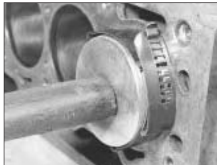
9.19 Fitting a piston/connecting rod
