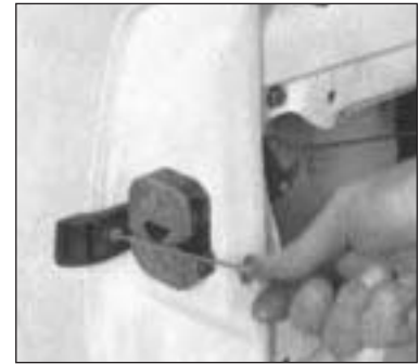
Fig. 12.11 Removing door handle fixing screw (three-door model) (Sec 12)
