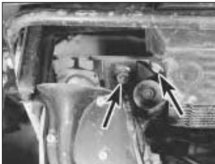
6B.25 Oil cooler mounting bolts (arrowed)
