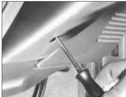
15.45A Undo the retaining screws . . .
