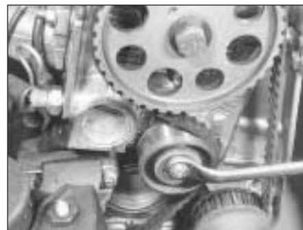
5B.9 Releasing the timing belt tensioner nut
