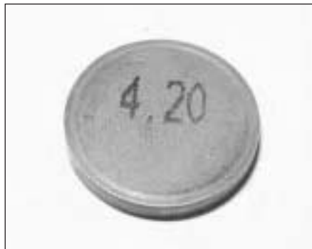
2B.25A Valve clearance shim showing thickness mark
