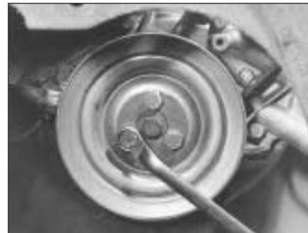
5B.7 Unscrewing the crankshaft pulley bolts
