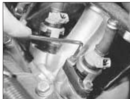
9C.80A Extracting a fuel injector screw
