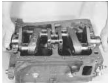
20.4B Lowering crankshaft into position
