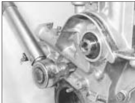
5D.12B Tightening an oil pump bolt
