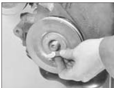
7B.34 Crankshaft pulley nut removal
