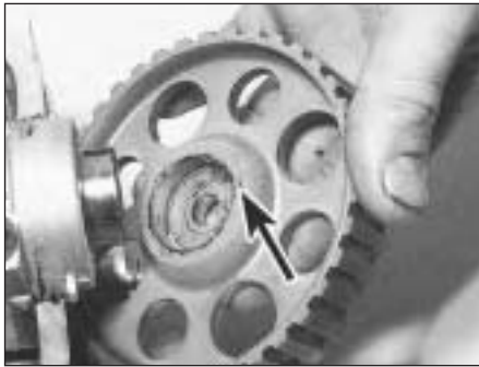
5B.22C Camshaft sprocket showing integral key (arrowed)
