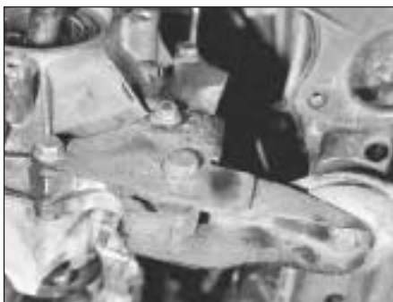
5C.26 Left-hand rear (lower) transmission mounting disconnected
