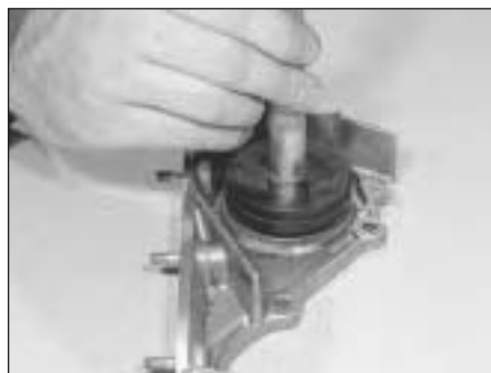
7B.140 Driving a new crankshaft front oil seal into its housing
