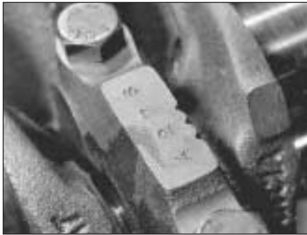
7C.69 Identification notches on No. 3 main bearing cap
