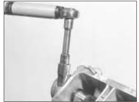
7B.85 Tightening a camshaft housing securing bolt
