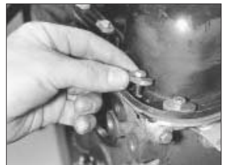
7B.166C . . . and insert the retaining bolts
