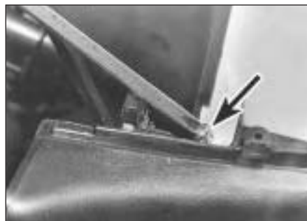
21.3 Removing instrument panel screw
