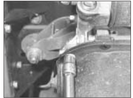
5B.63A Tightening a sump pan screw
