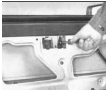
Fig. 12.6 Door glass mounting screw (Sec 12)
