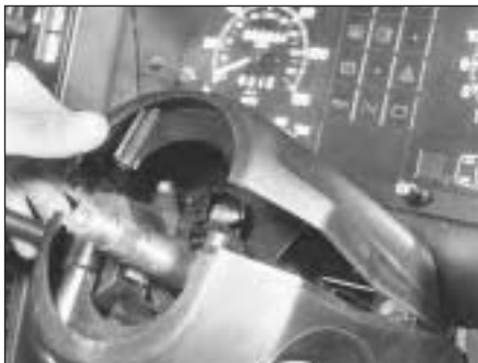
5.2 Removing steering column shrouds
