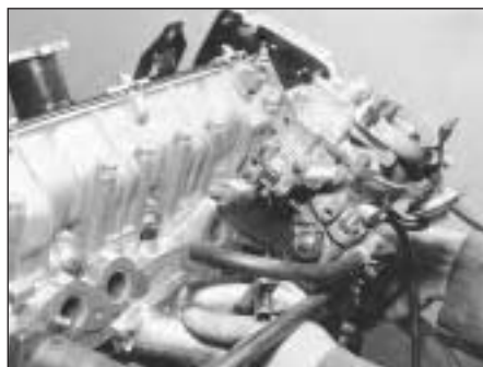
19.4C Fitting intake manifold complete with carburettor
