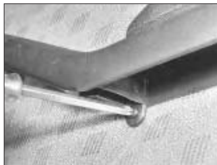
11.1A Removing an armrest screw
