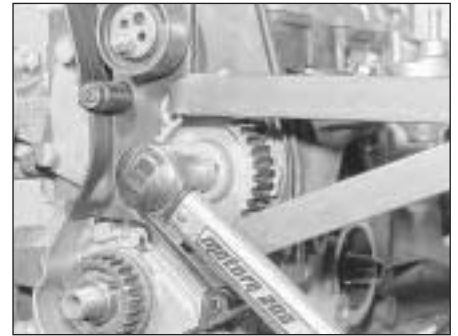
7B.46 Tightening the auxiliary shaft sprocket bolt
