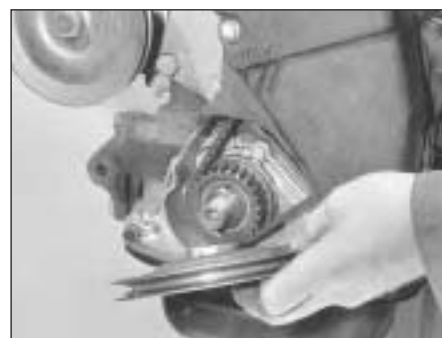
7B.35 Crankshaft pulley removal
