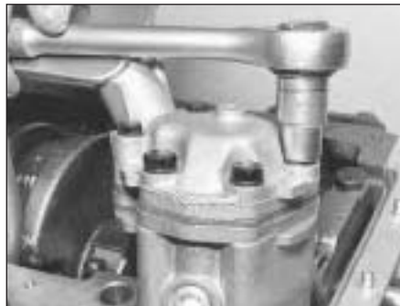
31.3 Bolting on the oil pump
