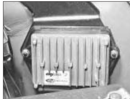
10.68 ECU location on the 1372 cc ie engine
