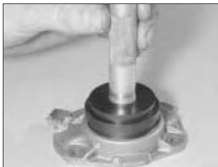
7C.53 Driving a new oil seal into the auxiliary shaft cover
