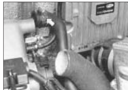
Fig. 13.56 Disconnecting the injector air cooling hoses and the supplementary air valve hose on the 1372 cc Turbo ie engine (Sec 9E)
