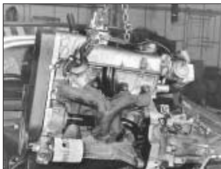
5C.34 Lifting out the engine and transmission
