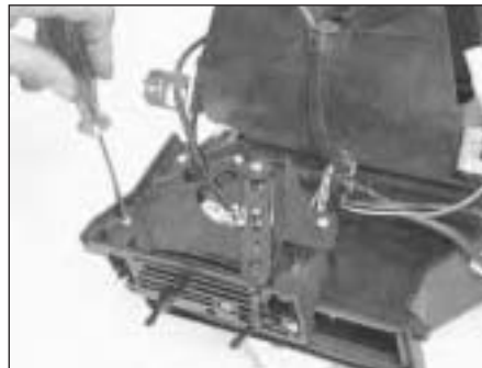
Fig. 2.9 Control lever platform screw (Sec 13)
