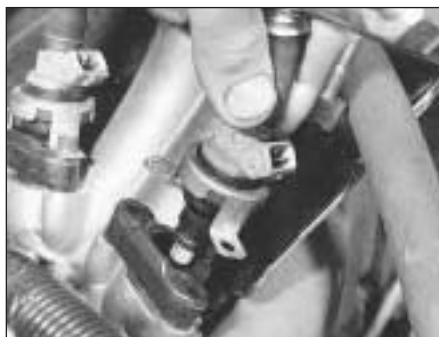
9C.80B Fuel injector removal
