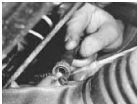
7C.32 Disconnecting the speedometer drive cable from the transmission
