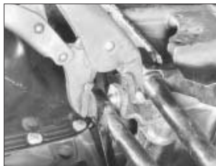
44.14 Connecting a gearchange rod ball cup
