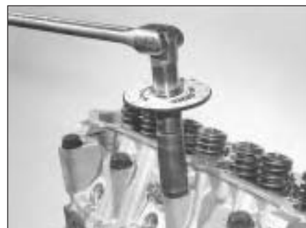
7B.121B . . . and then through the specified angle
