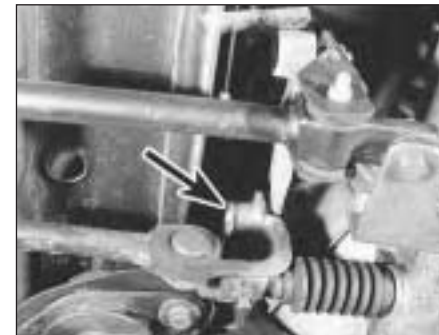
12A.6 Gearchange link rod spring clip (arrowed) on the 1301 cc Turbo ie engine
