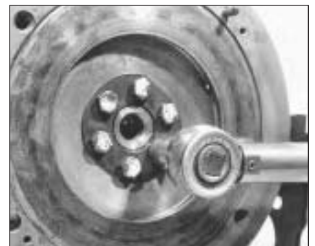
20.14 Tightening flywheel bolts
