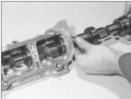
7B.93 Withdrawing the camshaft from its housing
