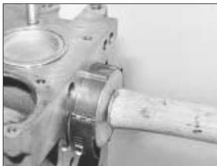
5B.97 Fitting a piston/connecting rod
