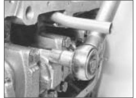
32.16 Tightening a big-end cap nut
