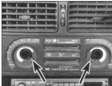
15.69A . . . undo the retaining screws (arrowed)
