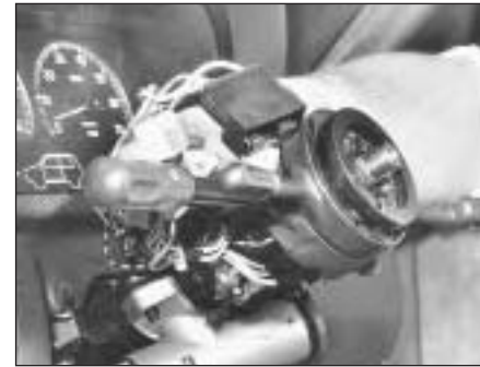
15.47B . . . and remove the column switch
