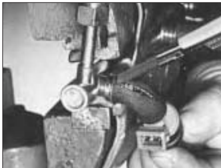
Fig. 13.61 Cutting free the hose from an injector on the 1372 cc Turbo ie engine (Sec 9E)
