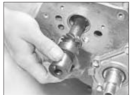
42.9 Fitting the auxiliary shaft
