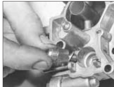
9B.26B Fuel inlet valve needle removal from the Weber 32 TLF carburettor
