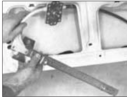
Fig. 12.10 Removing door window regulator (Sec 12)
