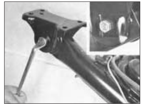
Fig. 11.9 Removing trailing arm pivot bolt (Sec 10)
