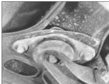
5B.107B Left-hand rear engine/transmission mounting
