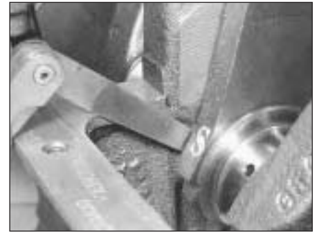
20.10 Checking crankshaft end float
