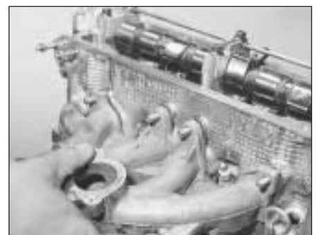
5D.25B Fitting the inlet manifold
