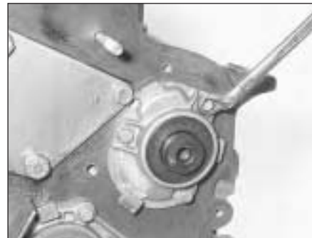
7C.55B . . . and tighten the securing bolts
