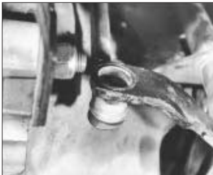
5C.24B Gearchange rod with ball socket connection
