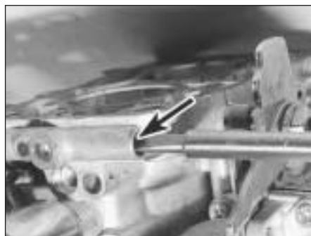
9B.36B . . . mixture screw (arrowed) on the Weber 30/32 DMTE carburettor
