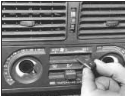
15.68 Remove the control knobs . . .
