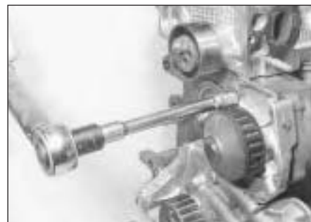
8A.17B Tightening the coolant pump bolts
