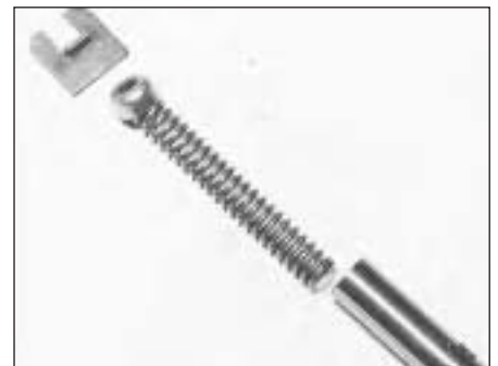
5B.72B Oil pump relief valve components
