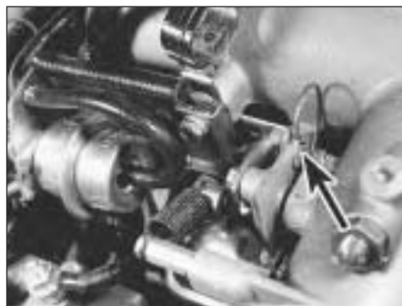
9C.99C Throttle cable nipple (arrowed) in throttle linkage cut-out
