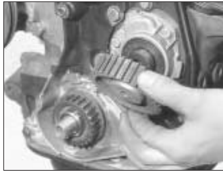
7B.45 Withdrawing the auxiliary shaft sprocket
