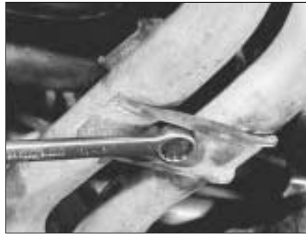
5C.23B Unscrewing the exhaust pipe lower support bracket bolt
