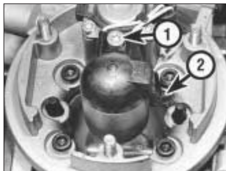
9D.49 Fuel injector unit sensor retaining screw (1). Also shown is the intake air temperature sensor (2)
