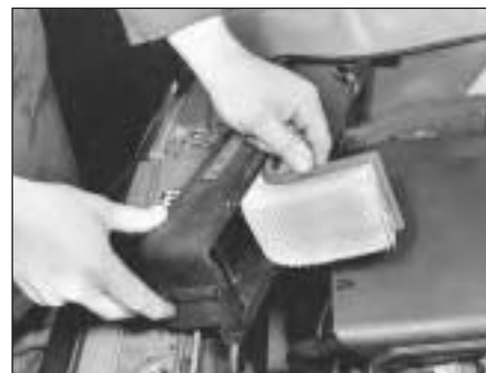
9D.17B . . . remove the cover and extract the element
