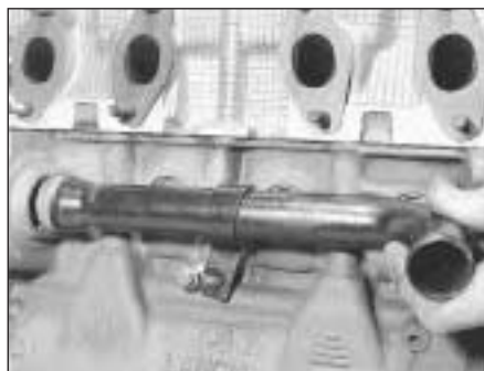
5D.30 Coolant distribution pipe
