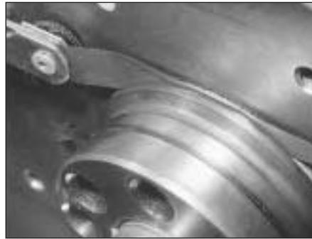
7C.70 Measuring crankshaft endfloat using feeler gauge method
