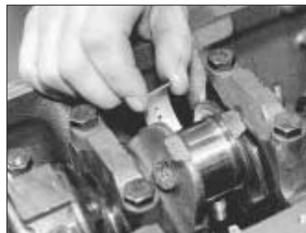
7B.195 Assemble the shell bearing to the connecting rod . . .
