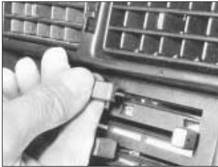
12.5 Pulling off heater control lever knob
