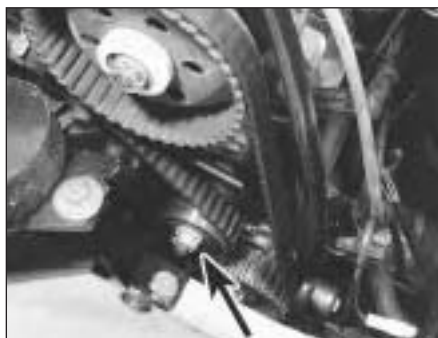
6B.20 Belt tensioner pulley locknut (arrowed)
