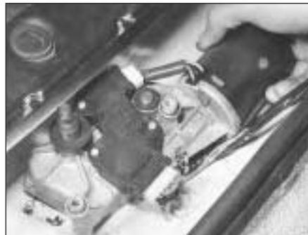
25.5B Removing windscreen wiper motor
