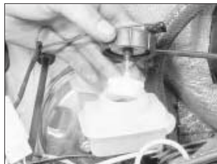
2.3 Fluid reservoir cap and float for warning switch
