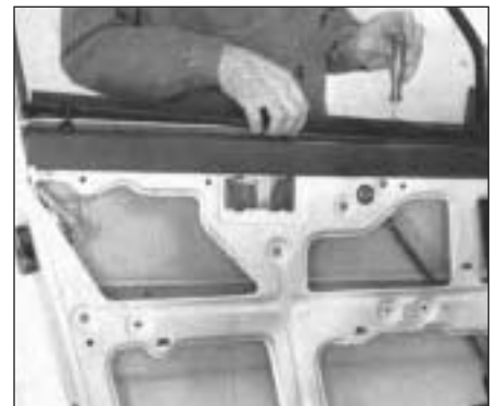
Fig. 12.7 Removing door weatherseal (Sec 12)
