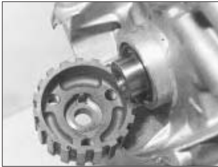
5D.16A Crankshaft sprocket showing integral key
