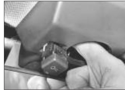
15.81 Roof-mounted spotlamp switch removal
