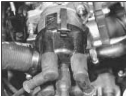
10.70 Ignition distributor and HT lead connections on the 1372 cc ie engine
