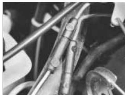
9B.37E Carburettor lead connectors on the Weber 30/32 DMTE carburettor
