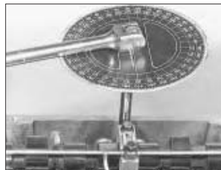
5B.52B Typical disc for angular tightening of cylinder head bolts
