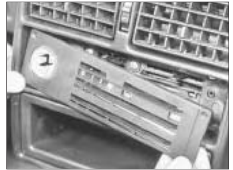
12.6B Removing heater control panel escutcheon
