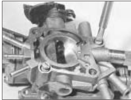
9B.26D Extracting the throttle valve block gasket from the Weber 32 TLF carburettor
