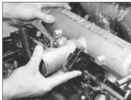
9C.73 Removing the inlet manifold
