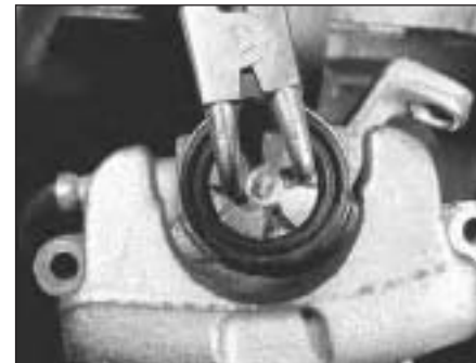
14B.28 Rotating a rear caliper piston
