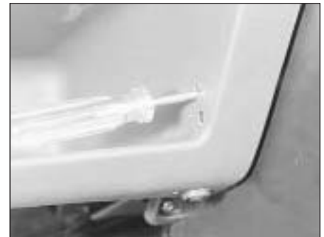
21.3 Removing screw (glovebox side) from centre console
