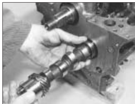
20.16A Fitting camshaft
