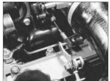
9C.99B Throttle cable (secondary section) and cross-shaft
