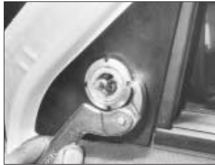
24.3 Mirror ring nut and C-spanner
