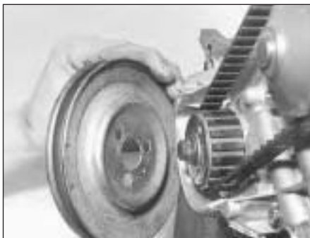
5D.22 Crankshaft pulley installation
