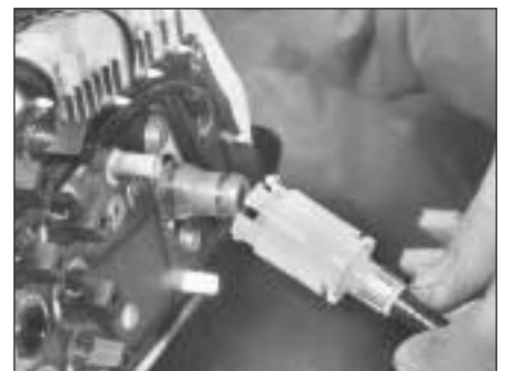
23.2 Speedometer cable connector at head
