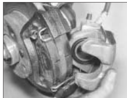
3.4 Removing the caliper unit
