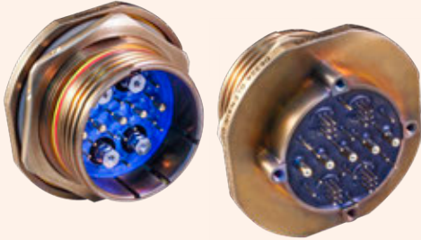
Harsh-environment marine bronze jam-nut connector, hybrid arrangement with #8 opto-electronic converter contacts and size #12 and #20 electrical contacts
