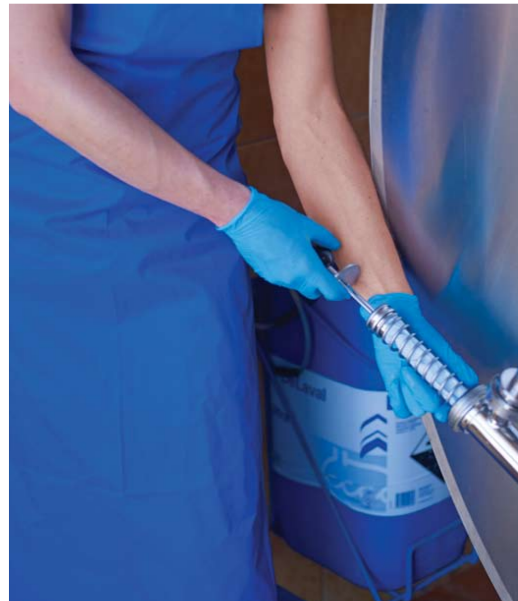
Image: Replacement of a milk filter
