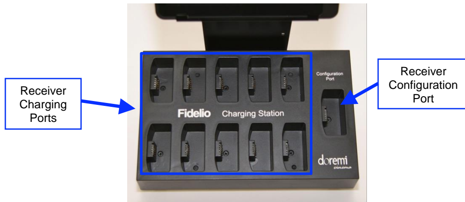
Figure 7: Fidelio Configuration/Charging Station - Top View
