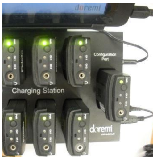
Figure 82: Fidelio Charging Station
