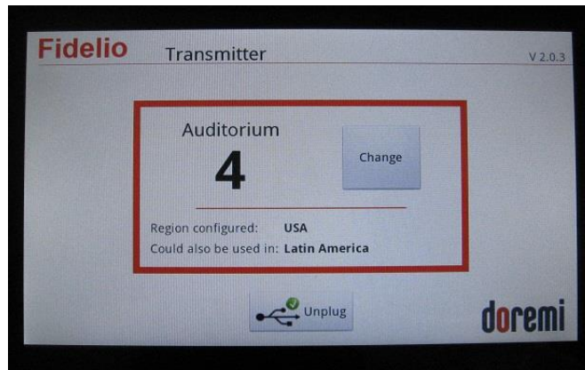
Figure 26: Transmitter Change Auditorium Screen
