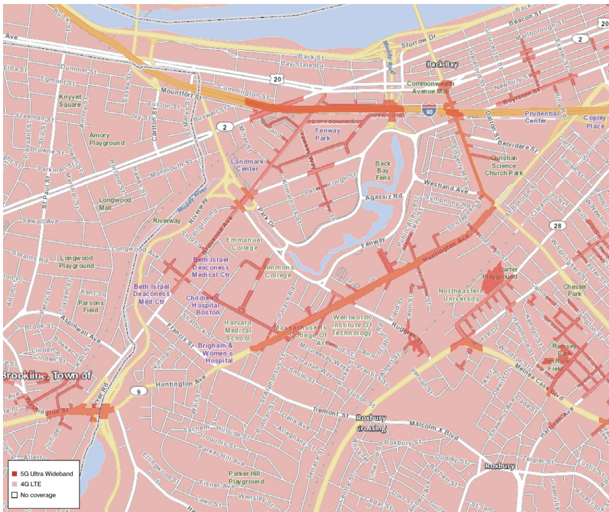
Figure 4 — This map showing Verizon's 5G Ultra Wideband coverage in Boston's Fenway/Kenmore area (as of November 2019) highlights the challenges of using higher frequency bands—coverage is extremely focused
