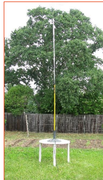
Figure 14 (at right) : WB6FRZ ground-plane antenna elevated 15 feet using a painter pole, umbrella stand, and table. Use guys if windy. Hanging it higher from the tree in the background would improve coverage.
