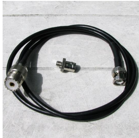
Figure 13 (at right) : Center adapter converts the HT connector to BNC which enables fast antenna swaps. Cable shown adapts from BNC to UHF (SO-239) although some cables end with a PL-259 instead.
