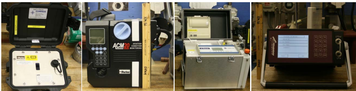
Figure 1. Parker Hannifin iOS, Parker Hannifin ACM20, Stanhope-Seta AvCount with SA1008-0 option, and PAMAS S40 Particle Counters (from left to right)
