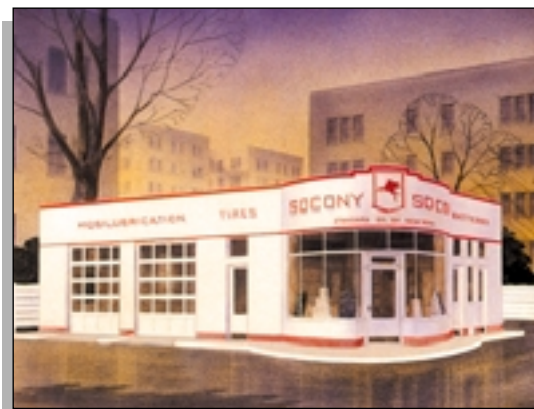
Figure 48: Frederick Frost developed this elegant porcelain enamel steel design for Socony-Vacuum in the late 1930s.
