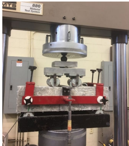
Figure 3-3 - Test setup for flexural strength measurement of beam specimens
