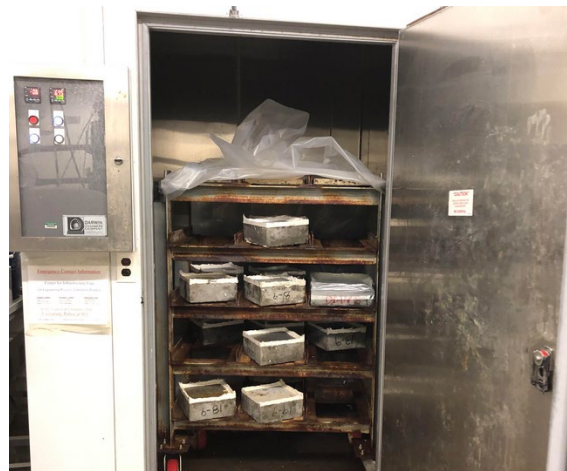
Figure 3-8 - Freeze-and-thaw chamber for deicing salt-scaling test
