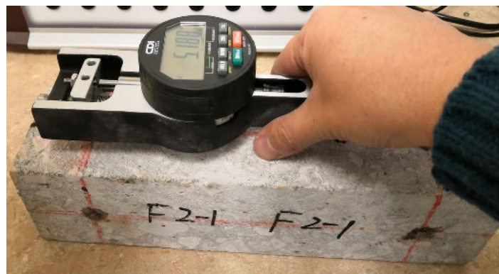
Figure 3-7 - Drying shrinkage testing
