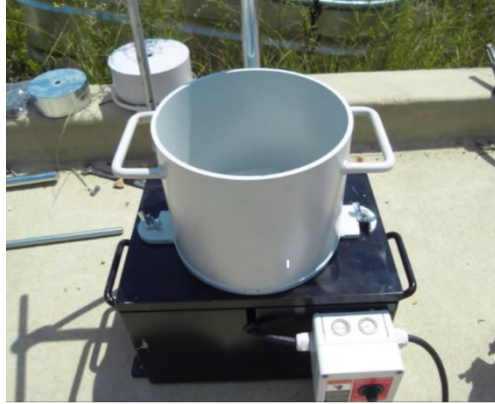
Figure 3-1 - Vebe test apparatus for determining consistency/density of fresh CCP
