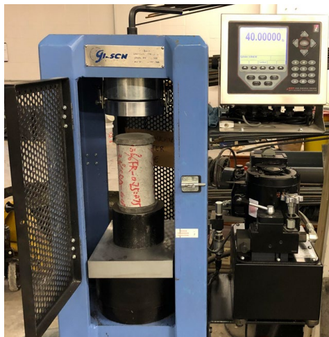
Figure 3-2 - Test setup for compressive strength measurement
