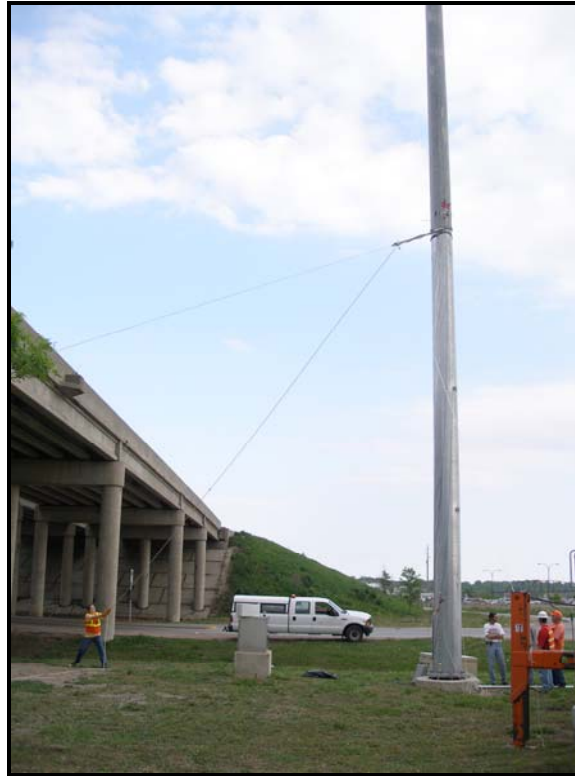
Figure 1.2 – Typical dynamic test of a retrofitted tower along I-29 in Sioux City, Iowa
