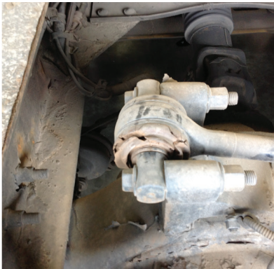
BUSHING MATERIAL IS TORN OR CRACKED
