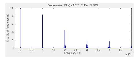
Fig.5. 40 Harmonic spectrum of unfiltered input phase current, IA
