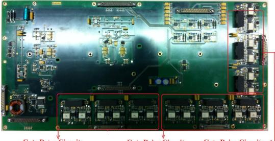
Gate Drive Circuits For Output Phase "a"
