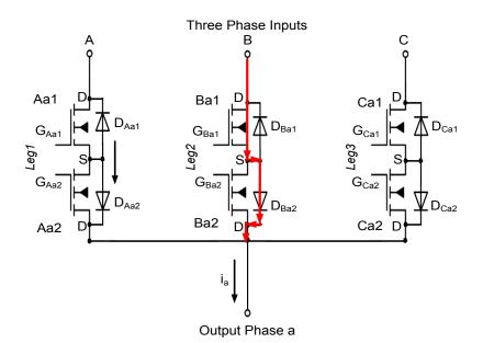
Fig.2. 25 Freewheeling current path in Leg2
