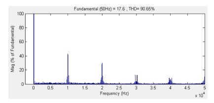
Fig.6. 9 Harmonic spectrum of output line-to-line voltage  $V_{ab}$  (f<sub>o</sub> = 50 Hz)
