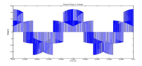
Fig.5. 34 Output phase "a" to neutral voltage,  $V_{an}$  (f<sub>o</sub> = 100 Hz)
