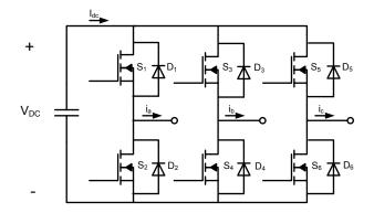
Fig.1. 2 Three-phase two-level voltage source inverter circuit topology
