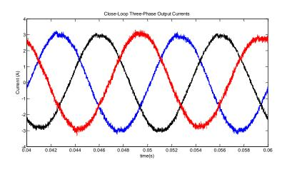
Fig.6. 26 Three-phase output currents ( $f_0 = 100 \text{ Hz}$ )
