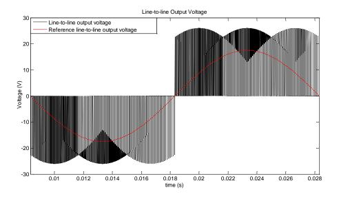
Fig.5. 24 Reference and observed output line-to-line voltage waveform,  $V_{ab}$
