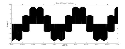
Fig.5. 11 Output phase "b" to neutral voltage,  $V_{bn}$  (f<sub>o</sub> = 50 Hz)
