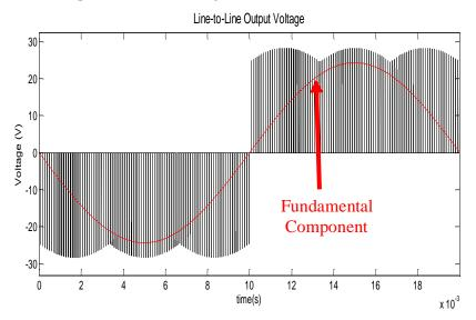
Fig.2. 4 Line-to-line output voltage waveform generated by direct matrix converter
