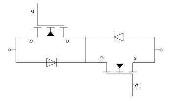
Fig.2. 17 Common drain AC switch configuration
