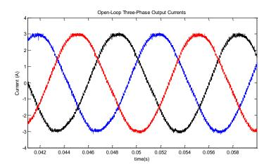
Fig.6. 15 Three-phase output currents ( $f_0 = 100 \text{ Hz}$ )
