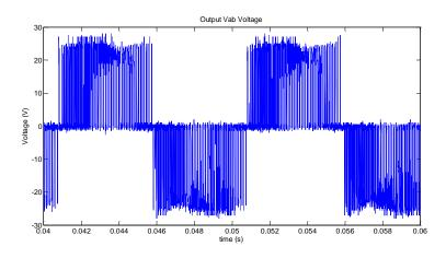
Fig.6. 13 Output line-to-line voltage  $V_{ab}$  (f<sub>o</sub> = 100 Hz)
