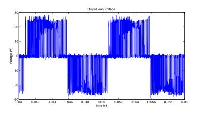
Fig.6. 24 Output line-to-line voltage  $V_{ab}$  (f<sub>o</sub> = 100 Hz)
