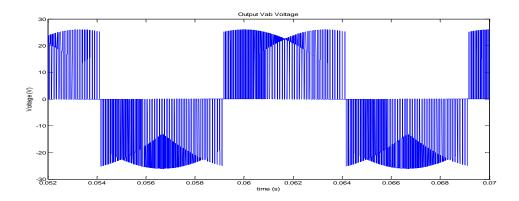
Fig.5. 20 Output line-to-line voltage  $V_{ab}$  (f<sub>o</sub> = 100 Hz)
