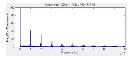
Fig.6. 14 Harmonic spectrum of output line-to-line voltage  $V_{ab}$  (f<sub>o</sub> = 100 Hz)
