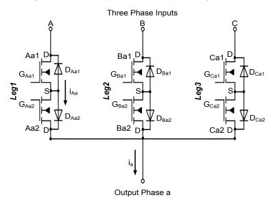
Fig.2. 24 One output phase structure
