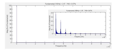
Fig.5. 38 Harmonic spectrum of output phase "a" current ( $f_0 = 100 \text{ Hz}$ )
