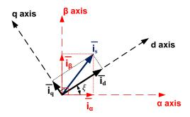
Fig. A. 3 D, q rotating reference frame
