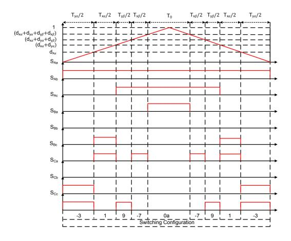
Fig.4. 16 Nine switching pulses for a carrier frequency of 10 kHz with double-sided switching pattern
