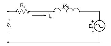
Fig.3. 3 Per-phase equivalent circuit of non-salient surface mounted permanent magnet synchronous machine
