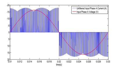
Fig.2. 7 Unfiltered input phase "A" current
