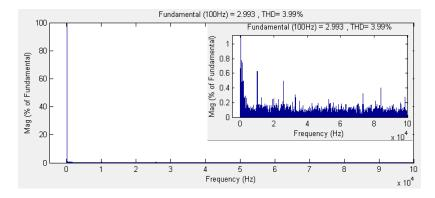
Fig.6. 27 Harmonic spectrum of the output phase "a" current ( $f_0 = 100 \text{ Hz}$ )
