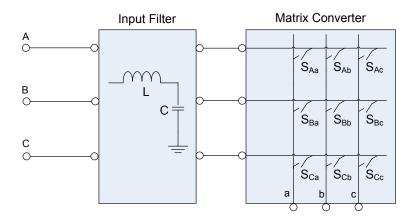
Fig.2. 3 Structure of matrix converter system
