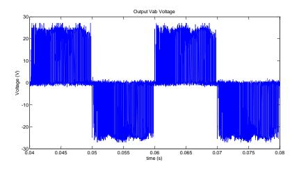
Fig.6. 8 Output line-to-line voltage  $V_{ab}$  (f<sub>o</sub> = 50 Hz)
