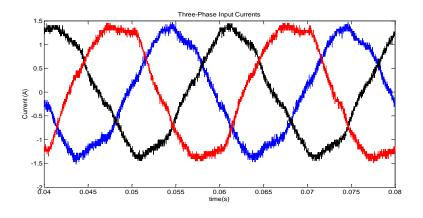
Fig.6. 32 Three-phase input currents
