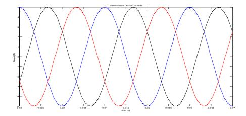
Fig.5. 45 Three-phase output currents ( $f_0 = 50 \text{ Hz}$ )
