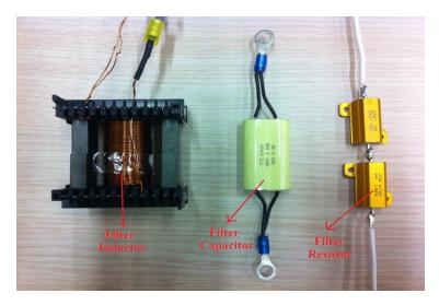
Fig.6. 2 One phase filter elements
