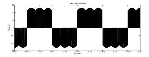
Fig.5. 14 Output line-to-line voltage  $V_{bc}$  (f<sub>o</sub> = 50 Hz)
