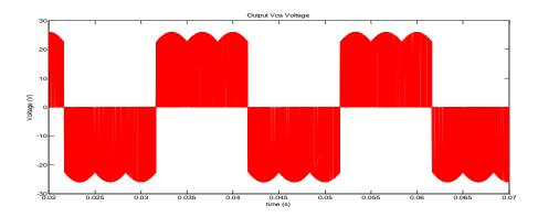
Fig.5. 15 Output line-to-line voltage  $V_{ca}(f_o = 50 \text{ Hz})$
