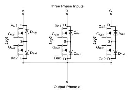
Fig.2. 23 One output phase structure of direct matrix converter
