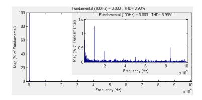
Fig.6. 16 Harmonic spectrum of the output phase "a" current ( $f_0 = 100 \text{ Hz}$ )
