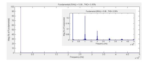
Fig.5. 18 Harmonic spectrum of the output phase "a" current ( $f_0 = 50 \text{ Hz}$ )
