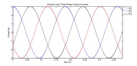
Fig.5. 58 Closed-loop three-phase output currents ( $f_0 = 5.5 \text{ Hz}$ )
