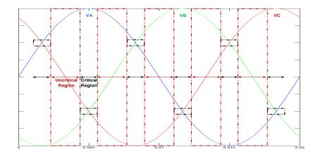
Fig.2. 30 Critical and uncritical intervals for detecting of input voltage polarities
