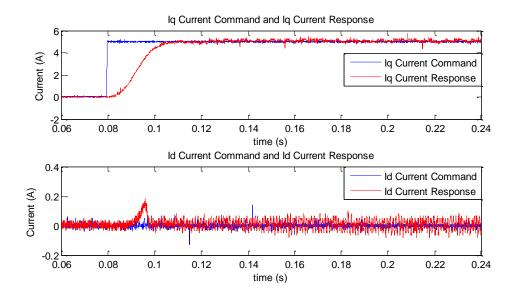
Fig.6. 17 Dynamic responses of the matrix converter circuit
