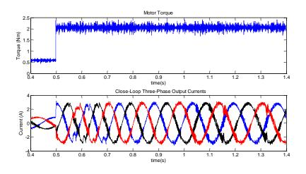
Fig.6. 36 Developed motor torque and converter output currents
