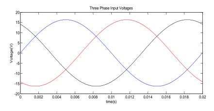
Fig.2. 6 Three-phase input voltages of direct matrix converter
