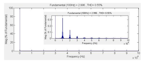
Fig.5. 23 Harmonic spectrum of the output phase "a" current ( $f_0 = 100 \text{ Hz}$ )
