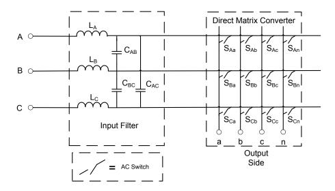
Fig.2. 12 Structure of three-phase to four-phase direct matrix converter
