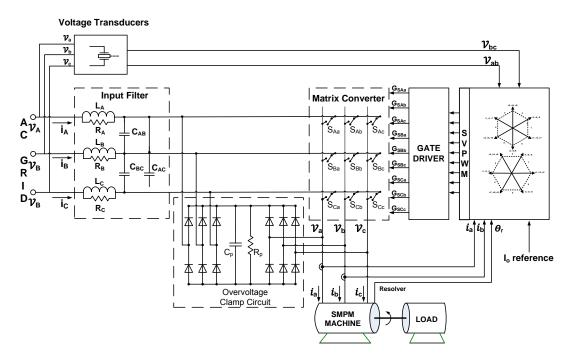
Fig.6. 1 Overall structure of the matrix converter circuit
