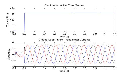
Fig.5. 59 Developed electromechanical motor torque and three-phase motor currents
