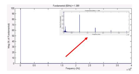
Fig.2. 10 Harmonic spectrum of filtered input phase A current ( $f_s = 10 \text{ kHz}$ )
