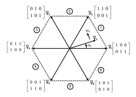
Fig.4. 11 Active output voltage space vectors, related sectors, and the reference output phase voltage vector,  $\overline{V_o}$  in complex plane
