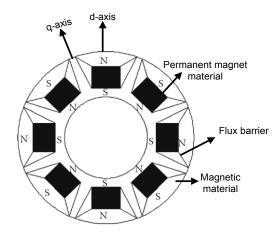
Fig.3. 2 Permanent magnet rotor construction using embedded magnets
