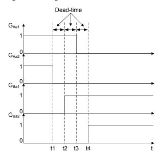
Fig.2. 26 Control signals of unidirectional switches
