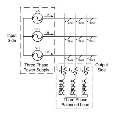
Fig.1. 7 Basic direct matrix converter circuit
