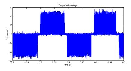
Fig.6. 34 Output line-to-line voltage  $V_{ab}$  (f<sub>o</sub> = 5.5 Hz)
