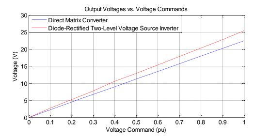
Fig.5. 49 Voltage linearity characteristics
