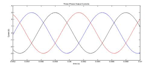
Fig.5. 22 Waveforms of the load currents ( $f_o = 100 \text{ Hz}$ )
