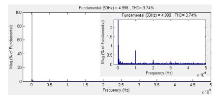
Fig.6. 11 Harmonic spectrum of the output phase "a" current ( $f_0 = 50 \text{ Hz}$ )
