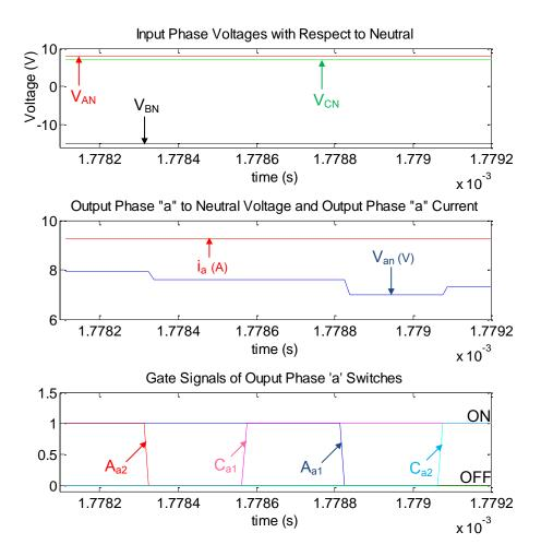
Fig.5. 25 Output current and voltage waveforms and the control signals of the semiconductor switches at a commutation instant
