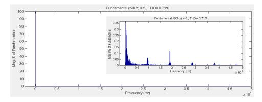
Fig.5. 46 Harmonic spectrum of output phase "a" current ( $f_0 = 50 \text{ Hz}$ )
