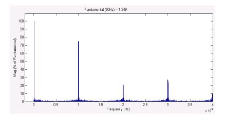
Fig.2. 8 Harmonic spectrum of unfiltered input phase A current ( $f_s = 10 \text{ kHz}$ )
