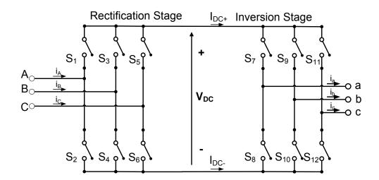
Fig.4. 7 Indirect matrix converter circuit
