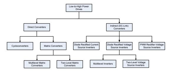
Fig.1.1 Classifications of converters low-to-high power drives
