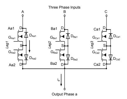
Fig.5. 26 Single phase output circuit structure
