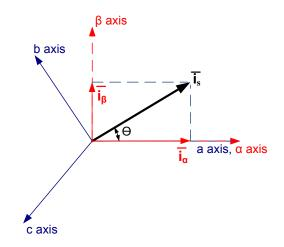
Fig. A. 1 Stator current representation in two co-ordinate stationary frame
