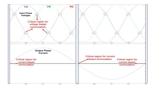
Fig.2. 31 Critical and uncritical intervals for output current direction and input voltage polarity based commutations
