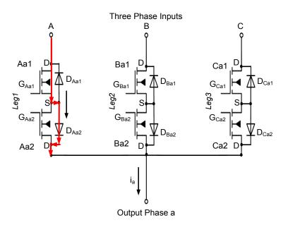
Fig.2. 27 Inductive current path in two step commutation
