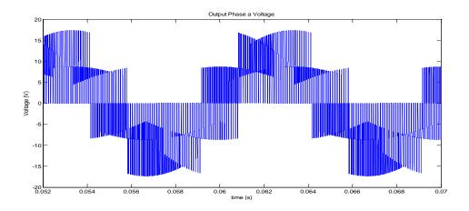
Fig.5. 19 Output phase "a" to neutral voltage,  $V_{an}$  (f<sub>o</sub> = 100 Hz)
