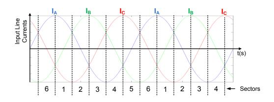
Fig.4. 9 Relationships between the input line current waveforms and the sectors in time domain
