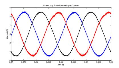
Fig.6. 21 Three-phase output currents at 50 Hz
