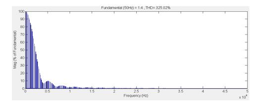
Fig.5. 48 Harmonic spectrum of input phase "A" current, IA
