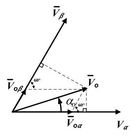
Fig.4. 13 Reference phase voltage vector construction
