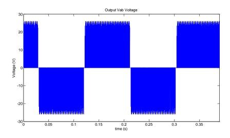
Fig.5. 57 Output line-to-line voltage,  $V_{ab}$  (f<sub>o</sub> = 5.5 Hz)
