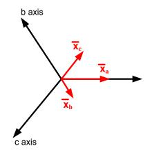
Fig.4. 3 Three variables of balanced three-phase system (  $\overline{x_a}, \overline{x_b}, \overline{x_c}$  )
