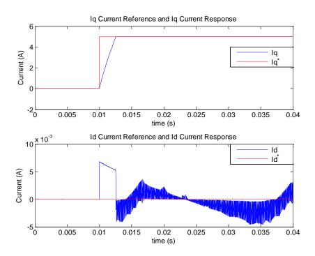
Fig.5. 54 Dynamic responses of d-axis  $(i_d)$  and q-axis  $(i_q)$  currents
