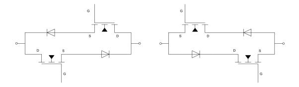
Fig.2. 18 Anti-parallel series diode-MOSFET configuration
