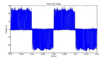
Fig.6. 19 Output line-to-line voltage  $V_{ab}$  (f<sub>o</sub> = 50 Hz)
