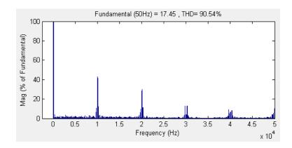
Fig.6. 20 Harmonic spectrum of output line-to-line voltage  $V_{ab}$  (f\_{o} = 50 Hz)  $\,$
