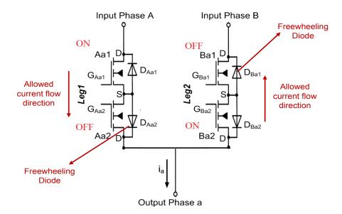
Fig.2. 29 Allowed current directions ( $\mathcal{V}_B > \mathcal{V}_A$ )
