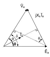
Fig.3. 4 Phasor diagram of the non-salient SMPM machine
