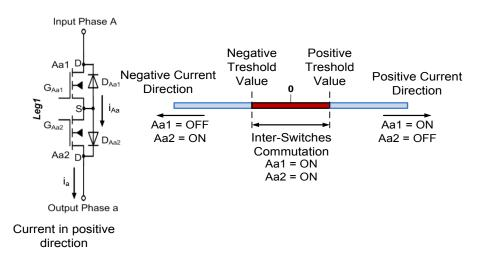
Fig.2. 28 Inter-Switches Commutation
