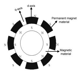
Fig.3. 1 Permanent magnet rotor construction using surface mounted magnets
