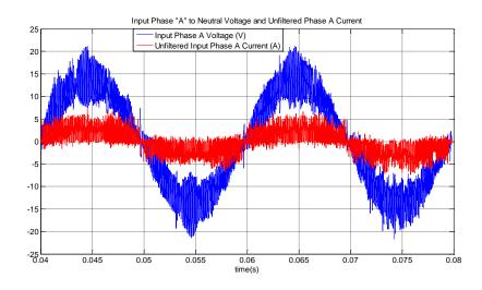
Fig.6. 28 Input phase "A" to neutral voltage, VAN and unfiltered input current, IA
