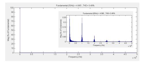
Fig.5. 33 Harmonic spectrum of output phase "a" current ( $f_o = 50 \text{ Hz}$ )
