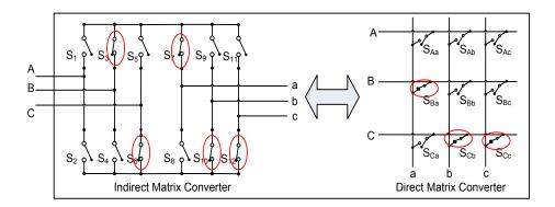
Fig.2. 14 An equivalent switching combination of direct and indirect matrix converter
