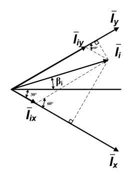
Fig.4. 10 Reference phase current vector construction
