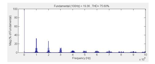
Fig.5. 21 Harmonic spectrum of output line-to-line voltage  $V_{ab}$  (f<sub>o</sub> = 100 Hz)
