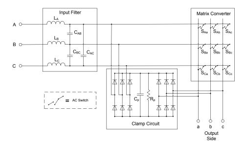
Fig.2. 19 The use of clamp circuit in direct matrix converter
