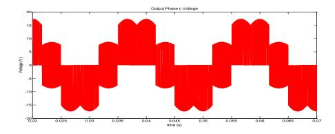
Fig.5. 12 Output phase "c" to neutral voltage,  $V_{cn}$  (f<sub>o</sub> = 50 Hz)
