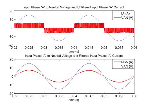
Fig.5. 39 Unfiltered and filtered input phase "A" current vs. input phase "A" voltage,  $V_{AN}$
