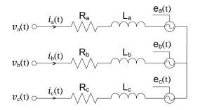
Fig.5. 51 Simulation model of the stator windings
