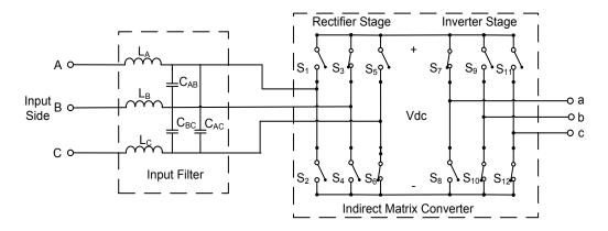
Fig.2. 13 Indirect three-phase to three-phase matrix converter
