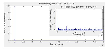
Fig.6. 22 Harmonic spectrum of the output phase "a" current ( $f_0 = 50$  Hz)
