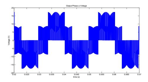
Fig.5. 29 Output phase "a" to neutral voltage,  $V_{an}$  (f<sub>o</sub> = 50 Hz)
