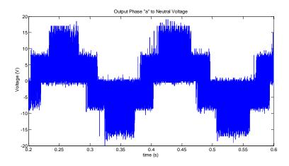
Fig.6. 33 Output phase "a" to neutral voltage,  $V_{an}$  (f<sub>o</sub> = 5.5 Hz)
