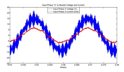
Fig.6. 30 Input phase "A" to neutral voltage,  $V_{AN}$  and filtered input current,  $I_A(f_i = 50 \text{ Hz})$
