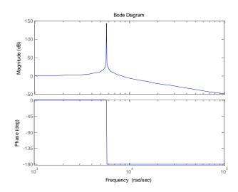
Fig.5. 4 Magnitude and phase plot of the LC filter without damping resistor
