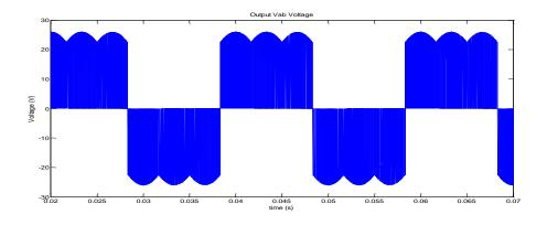
Fig.5. 13 Output line-to-line voltage  $V_{ab}$  (f<sub>o</sub> = 50 Hz)
