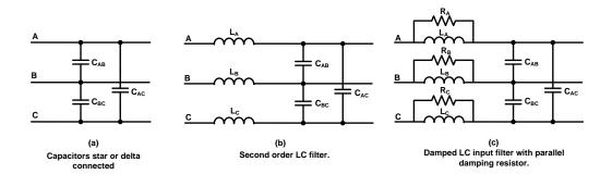
Fig.5. 1 Input filter configurations used for matrix converter input filters
