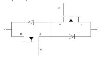
Fig.2. 16 Common source AC switch configuration
