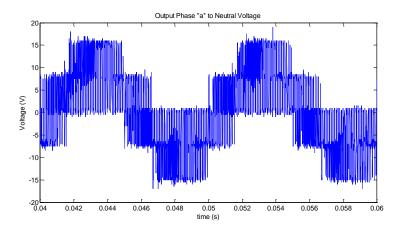
Fig.6. 12 Output phase "a" to neutral voltage,  $V_{an}$  (f<sub>o</sub> = 100 Hz)
