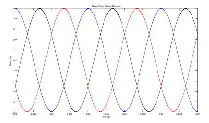
Fig.5. 31 Close-loop output currents ( $f_o = 50 \text{ Hz}$ )
