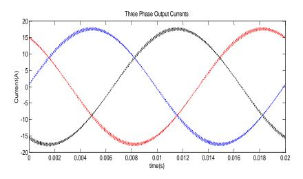
Fig.2. 5 Three-phase output currents of a direct matrix converter
