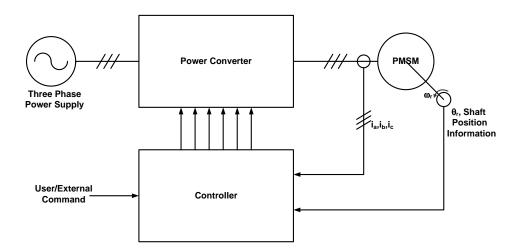
Fig.2. 1 PMSM drive basic architecture
