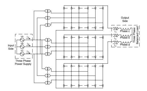
Fig.1. 6 Phase-controlled thyristor-based three-phase to three-phase cycloconverter
