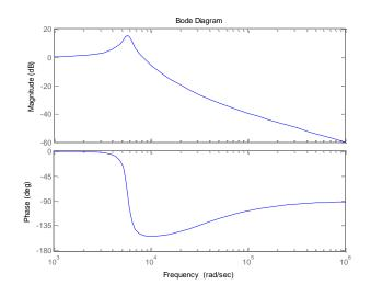
Fig.5. 3 Magnitude and phase plot of the LC filter with  $R_f = 94$  Ohm
