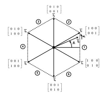
Fig.4. 8 Active current vectors, related sectors, and the reference phase current vector  $\overline{I_i}$  in complex plane
