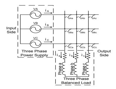
Fig.4. 1 Simplified three-phase to three-phase matrix converter
