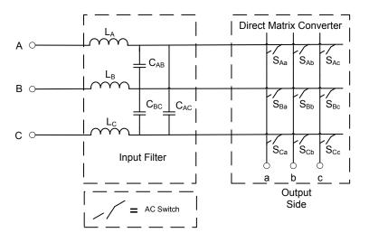
Fig.2. 11 Structure of direct matrix converter
