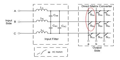
Fig.2. 21 Line to line short circuit condition
