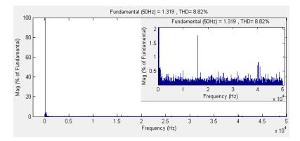
Fig.6. 31 Harmonic spectrum of the filtered input phase "A" current ( $f_i = 50 \text{ Hz}$ )
