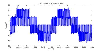
Fig.6. 23 Output phase "a" to neutral voltage,  $V_{an}$  (f<sub>o</sub> = 100 Hz)
