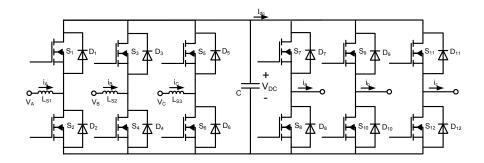
Fig.1. 5 Back to back voltage source converter
