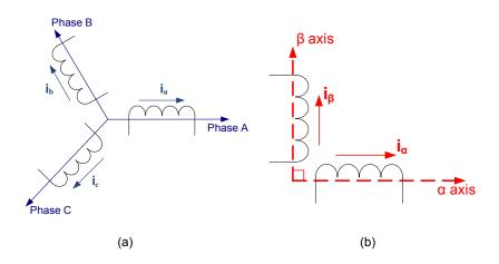
Fig. A. 2 (a) Three-phase balanced windings and (b) its two axes equivalent
