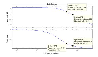
Fig.5.9 Theoretical magnitude and phase plots of load transfer function
