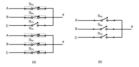
Fig.4. 5 Switching constraints (a) possible short circuit states at input terminal (b) open circuit state at output terminals
