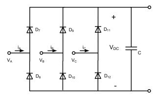
Fig.1. 3 Diode rectifier stage
