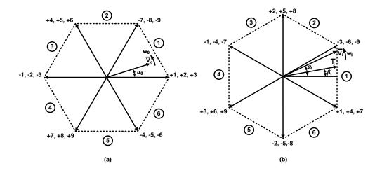
Fig.4. 14 (a) Voltage space vectors (b) current space vectors
