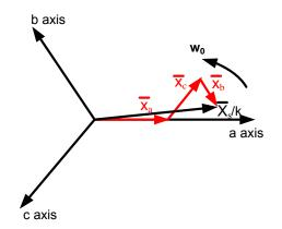
Fig.4. 4 Space vector  $\overline{X_s}$  and its components
