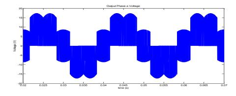
Fig.5. 10 Output phase "a" to neutral voltage,  $V_{an}$  (f<sub>o</sub> = 50 Hz)
