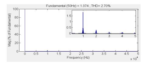
Fig.5. 41 Harmonic spectrum of filtered input phase current, IA
