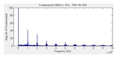
Fig.6. 25 Harmonic spectrum of output line-to-line voltage  $V_{ab}$  (f\_{o} = 100 \ Hz)
