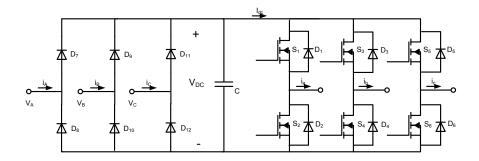
Fig.1. 4 Diode rectifier based VSI
