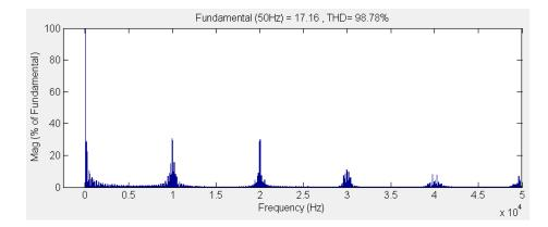
Fig.5. 32 Harmonic spectrum of output line-to-line voltage  $V_{ab}$  (f<sub>o</sub> = 50 Hz)
