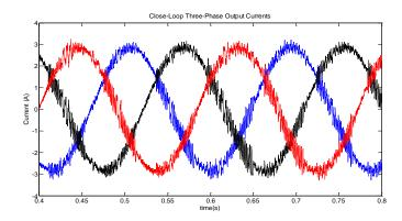
Fig.6. 35 Three-phase output currents ( $f_0 = 5.5 \text{ Hz}$ )
