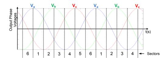
Fig.4. 12 Time domain relationship between the output phase voltage waveforms and sectors
