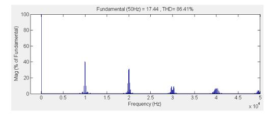
Fig.5. 16 Harmonic spectrum of output line-to-line voltage  $V_{ab}$  (f<sub>o</sub> = 50 Hz)
