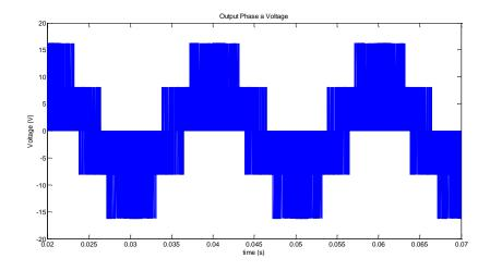
Fig.5. 42 Output phase "a" to neutral voltage,  $V_{an}$  (f<sub>o</sub> = 50 Hz)
