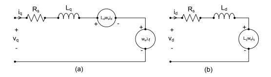
Fig.3. 6 Two-phase (d, q) equivalent model of SMPM synchronous machine
