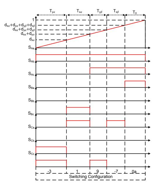
Fig.4. 15 Nine switching pulses for a carrier frequency of 10 kHz with single-sided switching pattern
