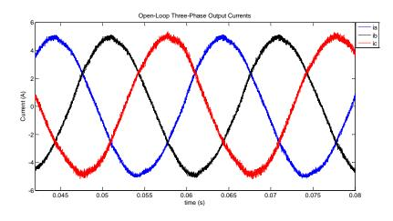
Fig.6. 10 Three-phase output currents ( $f_0 = 50 \text{ Hz}$ )
