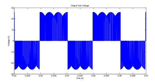
Fig.5. 30 Output line-to-line voltage  $V_{ab}~(f_{\rm o}\,{=}\,50~Hz)$
