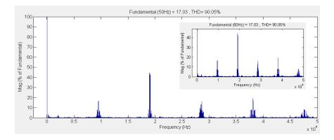
Fig.5. 44 Harmonic spectrum of output line-to-line voltage  $V_{ab}$  (f<sub>o</sub> = 50 Hz)
