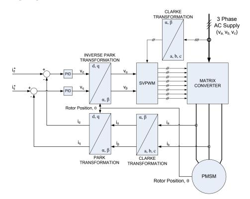
Fig.5. 50 Basic scheme of FOC for permanent magnet synchronous motor
