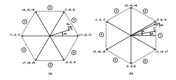
Fig.4. 6 (a) Output phase voltage vector (b) input line current vector hexagons
