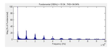
Fig.5. 36 Harmonic spectrum of output line-to-line voltage  $V_{ab}$  (f\_o = 100 Hz)
