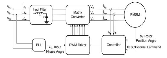
Fig.2. 2 Block diagram of PMSM drive system
