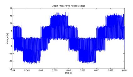
Fig.6. 7 Output phase "a" to neutral voltage,  $V_{an}$  (f<sub>o</sub> = 50 Hz)
