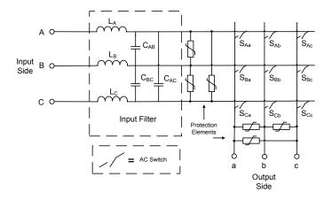
Fig.2. 20 Input/output varistor/suppressor diode protection scheme
