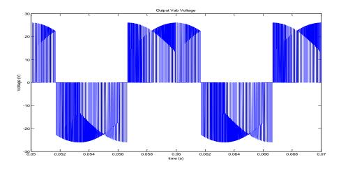
Fig.5. 35 Output line-to-line voltage  $V_{ab}$  (f<sub>o</sub> = 100 Hz)
