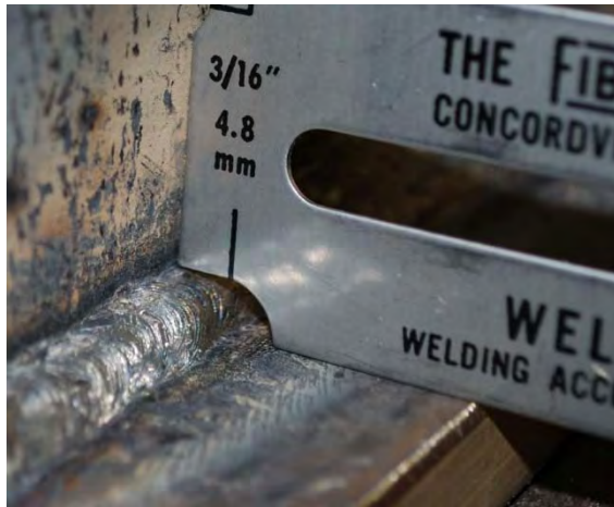
A 1/8" 7018 can potentially produce a 3/16" weld size with one pass and 5/16" with 3 passes.
