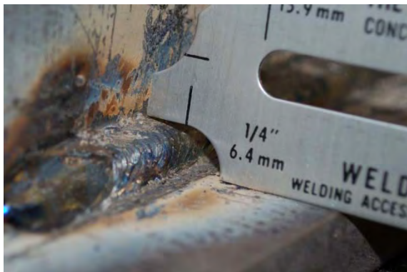
A 5/32" 7018 can potentially produce a 1/4" weld size with one pass and 3/8" with 3 passes.
