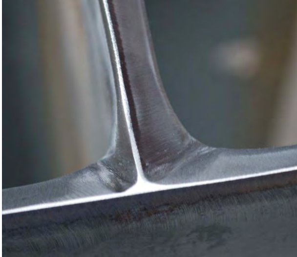
45 degree bevel on inside of flange and right side of web, inspection of the bevel angle.
