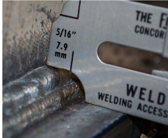
A 1/8" 7018 can potentially produce a 3/16" weld size with one pass and 5/16" with 3 passes.
