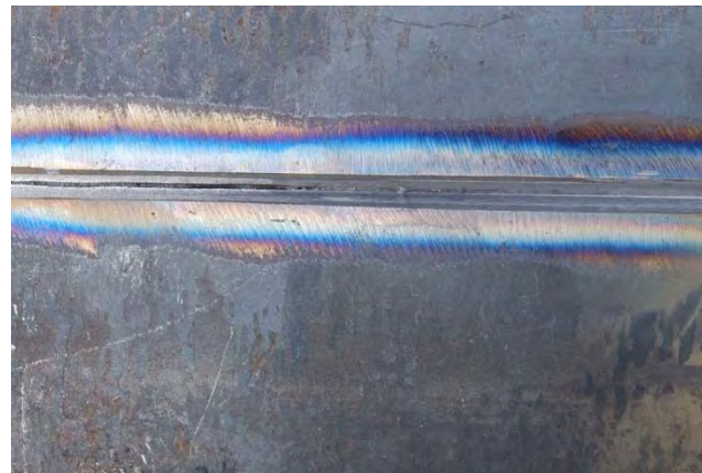
Back gouge on the right is Adequate, left is not.
