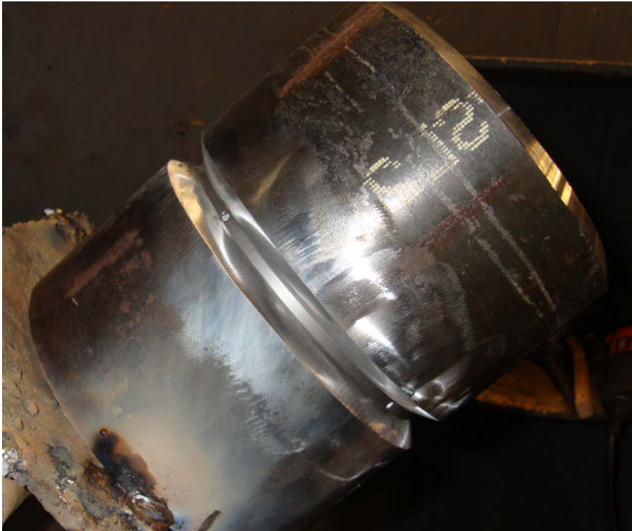
Coupon fit-up (place the splice in backing ring at the top).
