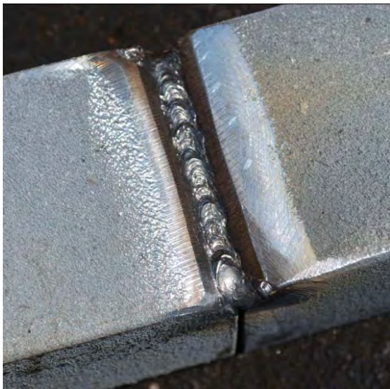
Each pass is cleaned.
