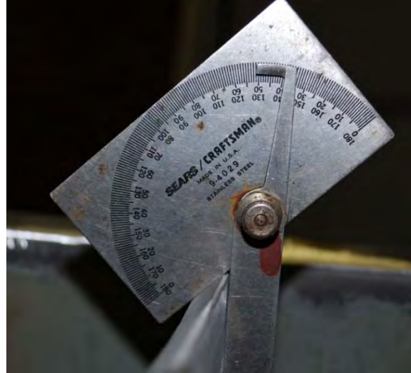
45 degree bevel on inside of flange and right side of web, inspection of the bevel angle.
