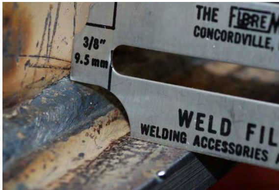
A 5/32" 7018 can potentially produce a 1/4" weld size with one pass and 3/8" with 3 passes.
