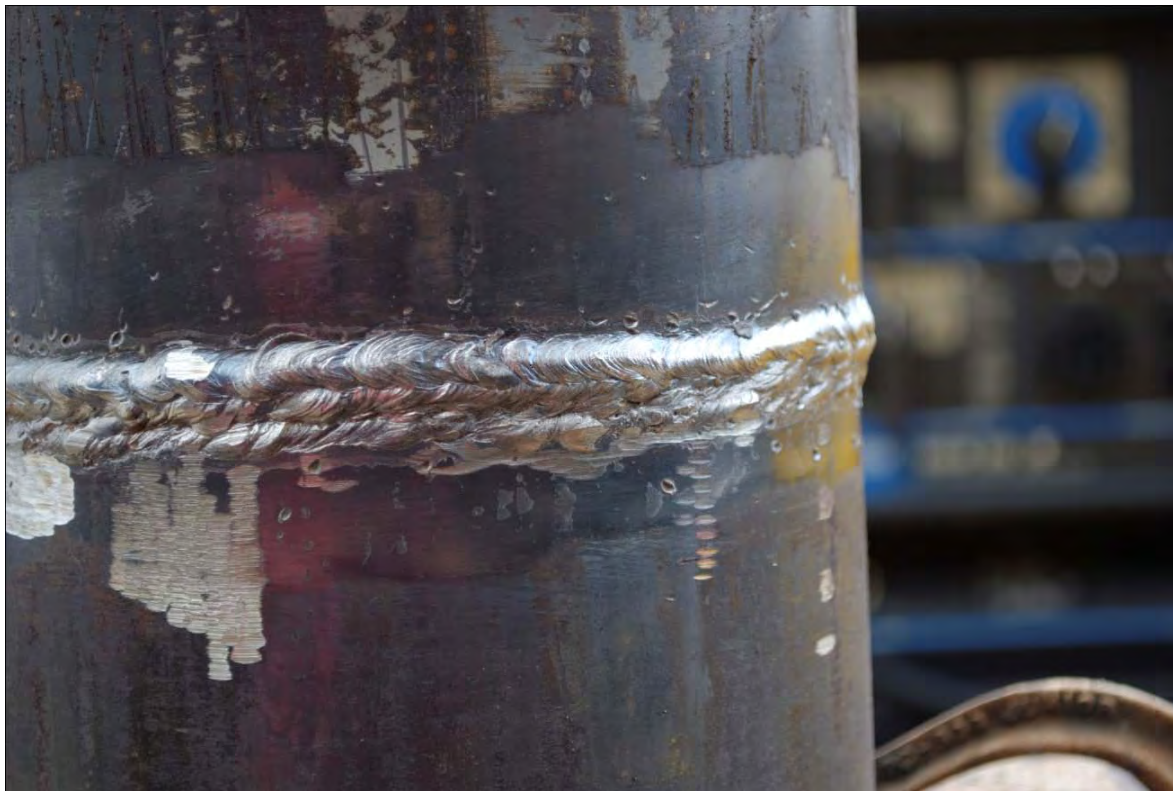
Acceptable weld (arc strikes removed by grinding)
