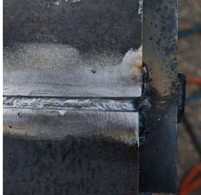
Each pass is cleaned.
