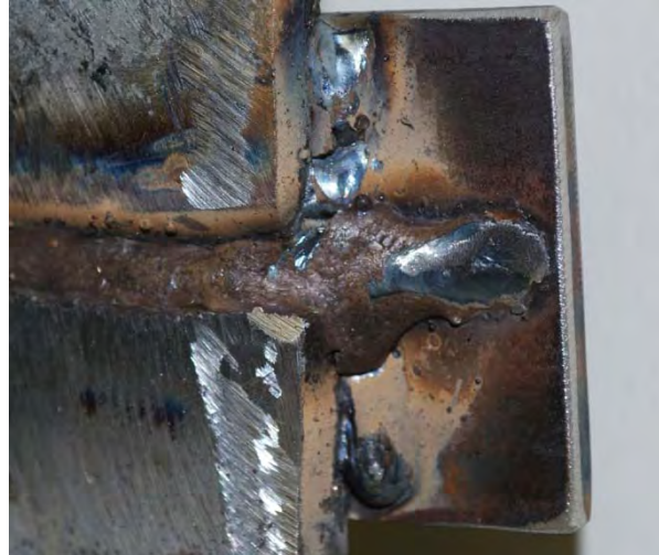
Runoff tabs are recommended but not required. The tabs make it easier to fill the groove at the end of the flanges.
