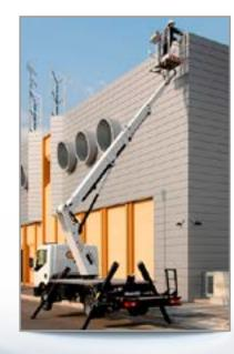
directional and proportional 4 sections electro-hydraulic functions
