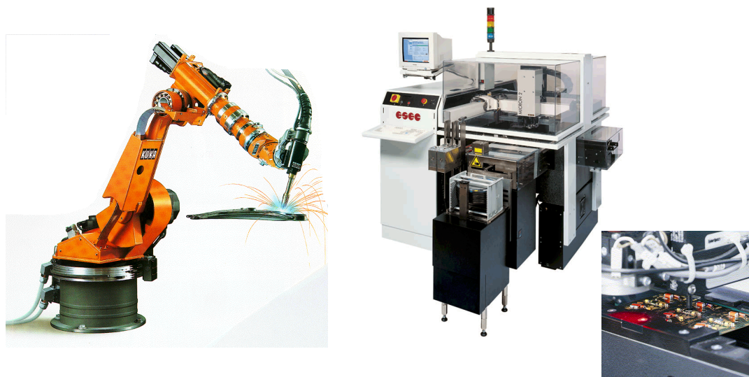
Fig 1.1 Picture of auto assembly plant spot welding robot in assembly line and surface mounter electronics arm during component assembly
