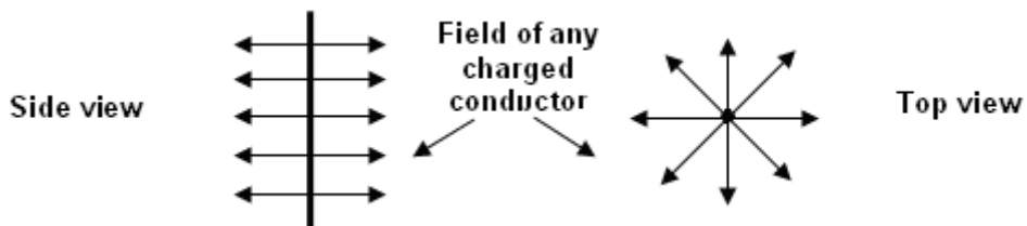
Fig.2 The electric field of any charged conductor
