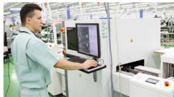
Inspecting solder quality on a 3D imaging system.
