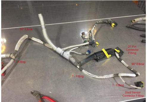
Figure 4 – Harness Clip Removal
