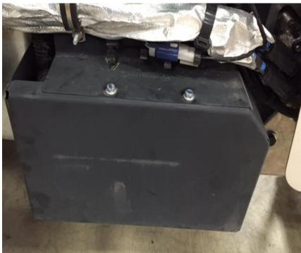
Figure 14 – ACM Cover Installation
