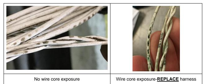
Figure 7 – Wire Harness Inspection
