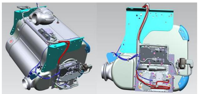
8. Carefully remove all convoluted tubing shown in red below. Reference Figure 6.
