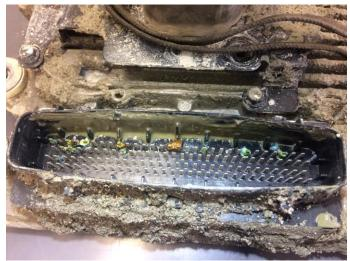
Figure 9 – ACM 21-pin and 120-pin Connector Inspection
