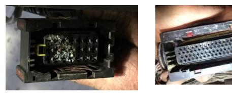
Figure 8 – ATS Harness 21-pin and 120-pin Connector Inspection
