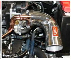
The air temp sensor, and hard pipe breather line have now been connected to the primary intake.
