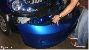
Prior to installing this cold air intake system, remove lower screws by the wheel well and the remaining plastic retaining clips. Once the plastic clips and screws have been removed, continue to slide the bumper off.
