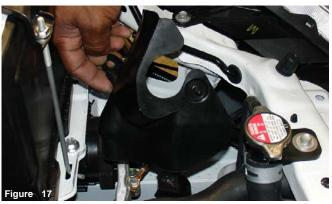
The plastic front cover is removed from the engine compartment.
