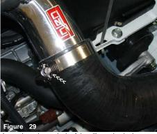
Approximately one inch of the silicone intake is pressed over the primary intake end. Once you have aligned the Primary intake to the silicone intake continue to fasten the Power clamp.
