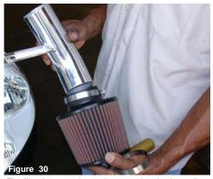
The filter is pressed over the secondary intake until the filter velocity stacks are flush with the intake. Once the filter is sitting flush, continue to tighten the filter neck clamp.
