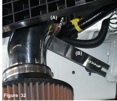
The secondary intake is pressed into the silicone intake (A). The intake bracket is aligned to the vibramount stud (B).
