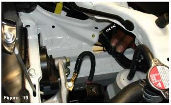
The harness is pulled away from the fender until a a clear path has been created for the silicone intake.
