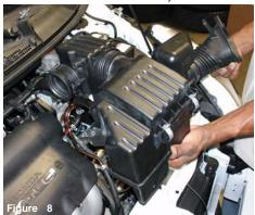
Once all lines and clamps have been removed from the air box cleaner, continue to lift and pull the air box cleaner from the engine compartment.
