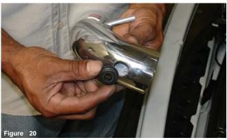
Insert the 1560 grommet into the pre-drilled hole located on the intake.
