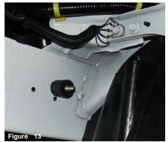
Screw the vibra-mount into pre-tapped hole until the vibra-mount can no longer be screwed in.
