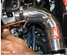
Insert the Crank case hard pipe into the 3"-8mm silicone hose located on the intake port.
