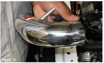
The sensor grommet is now sitting flush in the pre-drilled intake hole.
