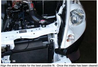
from all moving parts, continue to tighten all nuts, bolts and clamps. Periodically, check the fitment of the entire intake to prevent damage to the intake.
