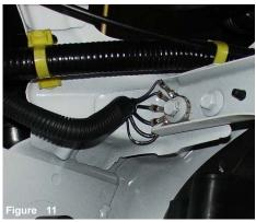
The have successfully relocated the ground wire connection.
