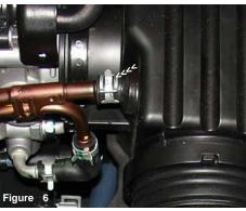
Using pliers, unhook the metal pressure clamp and pull the stem out from inside the air box cleaner.
