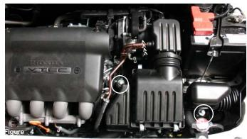
Unscrew the two bolts as shown above and loosen the clamp at the throttle body in order to remove the air box cleaner and duct.
