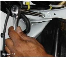
The 6mm screw is removed to relocate ground wire to the top cross member section as shown above.
