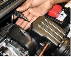
Lift the rear section of the air box cleaner and remove the air temperature sensor from the grommet.
