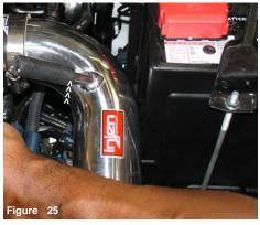
Press the 4"-10mm hose over the PCV hard line as shown above.
