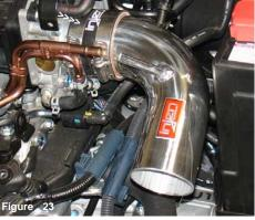
Press the primary intake into the throttle body hose as shown above, and semi-tighten the power-band.
