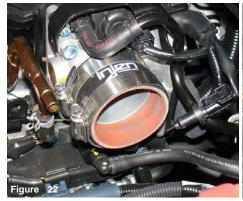
Press the straight hose over the throttle body and use two power-bands.
