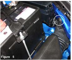
Pop the plastic head cap and remove the clip from the fender wall as shown above. Loosen the battery tie and push battery closer to the fuse box. This will allow more room between the battery and intake.
