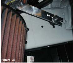
The m6 flange nut and fender washer is placed over the vibra-mount stud and the nut is tightened over the bracket.
