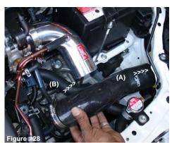
The silicone intake is inserted into the front opening between the head light and the harness location (A). The silicone intake is slipped into the opening until the top end is lined up to the primary intake. (B)
