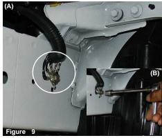
Ground wire to be removed from its stock location (A). Use a 10mm socket to loosen and remove the ground wire harness from the frame (B).
