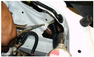
The harness clip is compressed and push through the fender in order to free the electrical harness.
