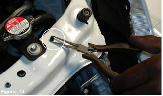
The first top clip is removed by compressing the tabs and pressing the pin through the hole.
