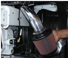
Insert the secondary assembled intake into the upper bumper section and into the end of the silicone hose.
