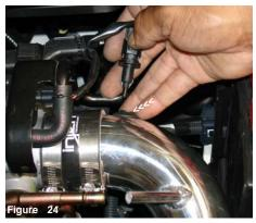
Press the air temperature sensor into the intake grommet, until it sits flush with the grommet.
