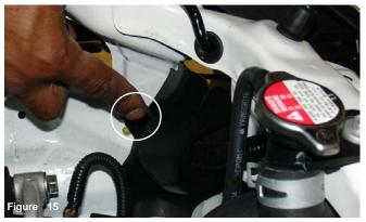
The second plastic clip is removed from the fender wall area.
