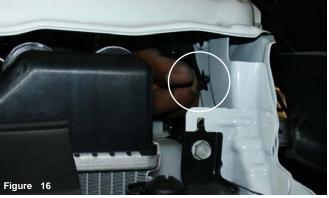
The inner plastic plug is removed from the main frame support.
