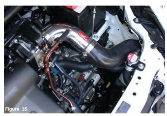
Top view of the cold air intake fully installed. The entire intake is now aligned prior to tightening any nuts and bolts.
