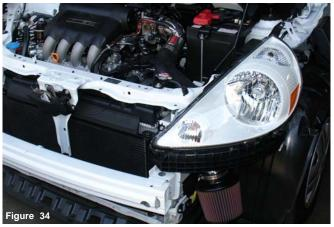
The assembled secondary intake and filter are now aligned and pressed into the silicone intake. The silicone power-band is now ready to be tightened over the secondary intake.
