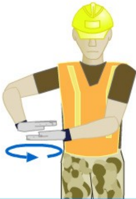
Cut, Fill, or Drag Road Point to road to be dragged or bladed, then rub palms together. Applies to scrapers, motor graders, and bulldozers.
