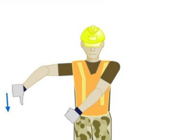
Lower Boom and Hold Load
