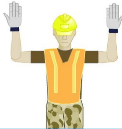
Maneuver Forward Slowly When maneuvering in close quarters or to move a foot or two at a time.
