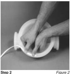
Starting at any point, place the Teflon® tape in the center of the diaphragm bead groove on the liquid chamber and press lightly on the tape to ensure that the adhesive holds it in place during assembly. Do not stretch the tape during placement in center of diaphragm bead groove. (*Figure 2*)
