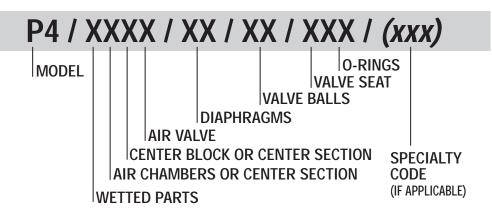
In the case where a center section is used instead of a center block and air chambers, the designation will be as follows: Acetal = LL
