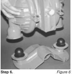
Lift liquid chambers and center section from intake manifold to expose intake valve balls and seats. Inspect ball cage area of liquid chamber for excessive wear or damage. (Figure 6)
