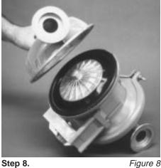
Lift liquid chamber away from center section to expose diaphragm and outer piston. (Figure 8)
