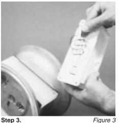
Lift away air valve assembly and remove air valve gasket for inspection (Figure 3). Replace if necessary.
