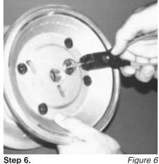
Remove pilot spool retaining snap ring on
