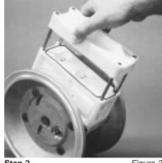
Step 2. Figure 2 Remove muffler plate and air valve bolts from air valve assembly (Figure 2) exposing muffler gasket for inspection. Replace if necessary.
