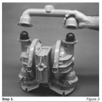
Remove the discharge manifold to expose the valve balls and seats. Inspect ball cage area of manifold for excessive wear or damage. (Figure 3)
