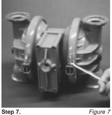
Remove one set of large clamp bands which secure one liquid chamber to the center section. (Figure 7)
