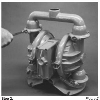
Utilizing a 7/6" wrench, remove the two small clamp bands that fasten the discharge manifold to the liquid chambers. (Figure 2)
