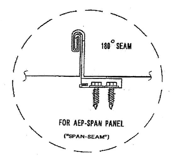
1. Metal Roof Deck Panels\* — No. 24 MSG min gauge coated steel, max width 16 in. Panels continuous over two or more spans. End lap to occur over purlins and to include End Lap Back-up Plate (Item 2B or 2C.) Ends of panels overlapped 6 in. Side laps to be tightened and crimped with a special motorized crimping machine at a minimum 45 degree angle with crimping process to include tabs of Panel Clips (Item 2). A bead of sealing compound may be used at panel end and side laps.
