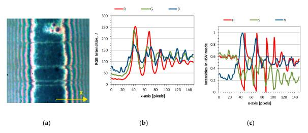
Figure 6. (a) Interferogram; (b) corresponding RGB and (c) HSV components on x-axis.
