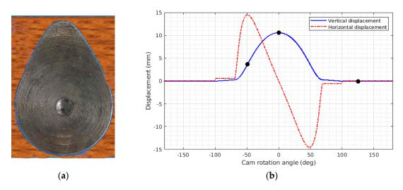
Figure 11. (a) Cam; (b) vertical and horizontal displacement of the contact zone.
