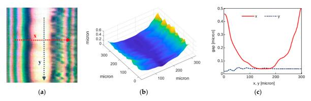
**Figure 14.** (**a**) Interferogram at  $125^{\circ}$ ; (**b**) fluid film 3D representation; (**c**) film thickness along the *x* and *y* axes shown in subfigure (**a**).
