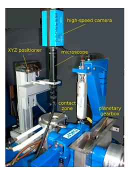
Figure 3. Picture of the optical system.
