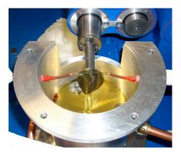
**Figure 2.** Picture of the top part of the measurement unit with the cover removed showing the cam mounted on the camshaft and the final part of the oil supply system.
