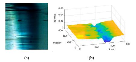
Figure 13. (a) Interferogram at 0° (cam nose); (b) fluid film 3D representation.
