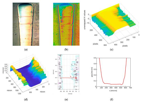
**Figure 12.** (a) Interferogram at the inversion point  $-49^{\circ}$ ; (b) corresponding enhanced image; (c) related 3D unwrapped signals; (d) 3D representation of the gap; (e) contour lines; (f) film thickness along the *x*-axis reported in subfigure (e).
