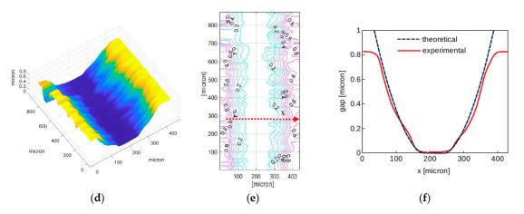
**Figure 10.** (a) Interferogram; (b) corresponding enhanced image and (c) related 3D unwrapped signals; (d) 3D representation of the gap; (e) contour lines; (f) comparison between theoretical and evaluated contact profile along the *x*-axis reported in subfigure (e)—static contact–load 30N.
