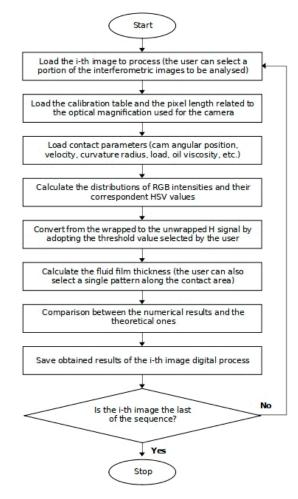
Figure 8. Block diagram of the program for the elaboration of interference images.
