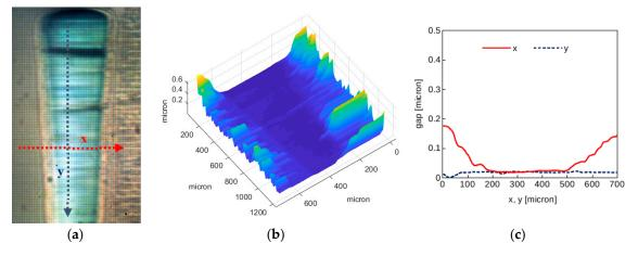
**Figure 15.** (a) Interferogram at  $-45^{\circ}$ ; (b) fluid film 3D representation; (c) film thickness along the *x* and *y* axes shown in subfigure (a).
