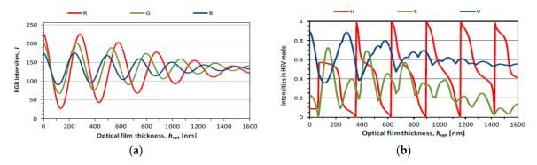
**Figure 5.** (**a**) Theoretical distributions of RGB intensities and (**b**) corresponding HSV values as function of the optical thickness.
