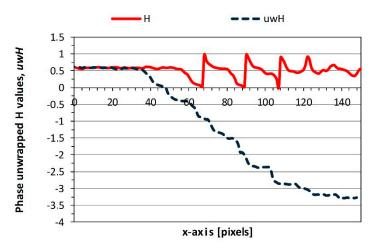
Figure 7. H and unwrapped signals uwH along a pixel row starting from the center of Figure 6a.
