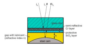
Figure 4. Basic principle of optical interferometry technique.
