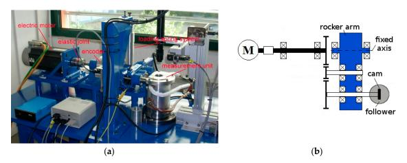
a disc, simulating a follower). The rig allows simultaneous measurements of contact force and film thickness. A picture and a schematic drawing of the apparatus are shown in Figure 1.
