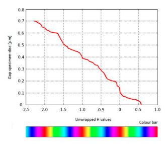
Figure 9. Calibration table and color bar for cam on glass disc in test basic configuration.
