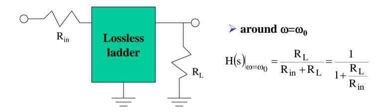
➤ In the passband, the transfer function can be very well controlled
