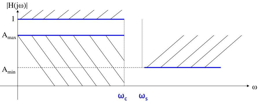
$A_{max} = A_p$  is the maximum attenuation in the passband  $A_{min} = A_s$  is the minimum attenuation in the stopband  $\omega_s - \omega_c$  is the Transition Width
