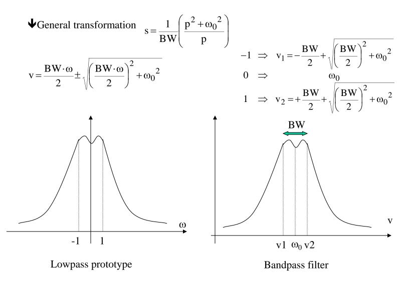
$\bullet$  The Lowpass to Bandpass transformation can also be applied to the elements
