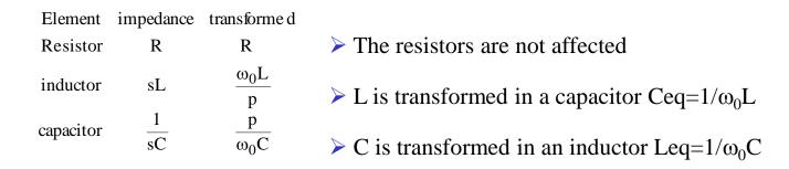
Example: Design a 1KHz HP-filter from a LP prototype.
