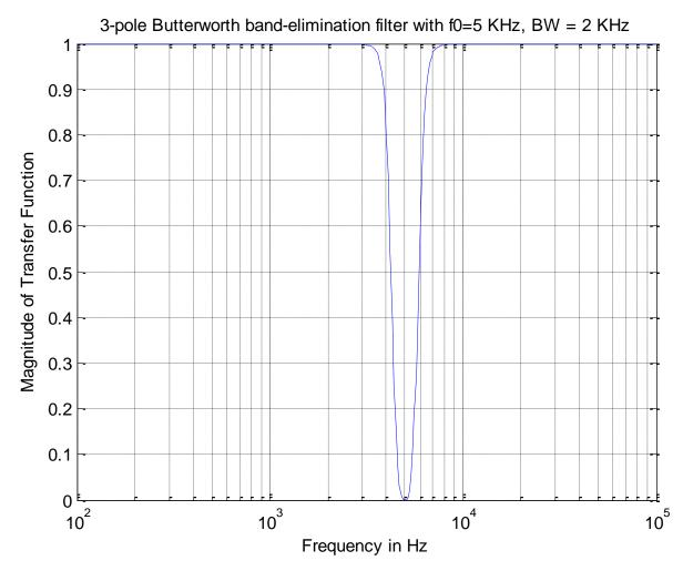
How to find the minimum order to meet the filter specifications ? The following functions in Matlab can help you to find the minimum order required to meet the filter specifications:
