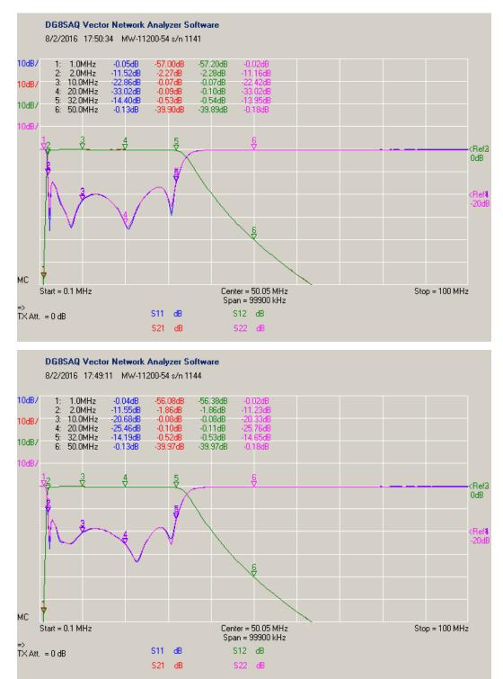
Figure 8 ~ Four sparameters for each of three filters are plotted in a rectangular format. The parameters and associated trace colors are indicated at the bottom of the display, and corresponding marker values are shown at upper-left. The filter model and serial number is shown above the marker table.
