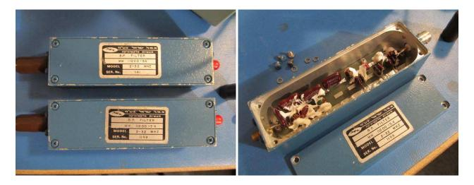
Figure 7 ~<u>Left</u>: Two obviously used AEL MW-11200-54 bandpass filters. Filter dimensions are 120 x 35 x 28 mm. <u>Right</u>: Interior view of the filter. Typical of AEL lumped element filters, parts are soldered to pads on a simple PCB and white rubbery adhesive is used to reduce microphonics and vibration effects. These high frequency filters use toroidal inductors but AEL filters for higher frequencies use single-layer air core coils. Images © 2016 W. Reeve
