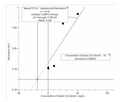
Figure D7. Concentration of (+)-catechin in unpasteurized beer filtered with 15 lbs SHG/100 bbls and 4 lbs PVPP/100 bbls.
