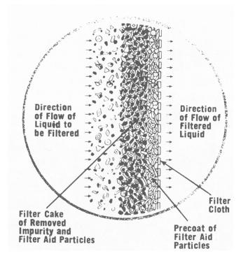
Figure 5. Filter Septum with the pre-coat and filter cake.
