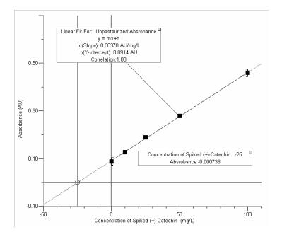
Figure D3. Concentration of (+)-catechin in unpasteurized beer filtered with 20 lbs SHG/100 bbls.
