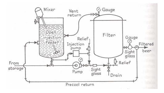
Figure 4. Diagram of a typical wire mesh kieselguhr filter From "A Textbook of Brewing," By Jean De Clerck, 1994, p. 464. Copyright 1957 by Chapman & Hall LTD
