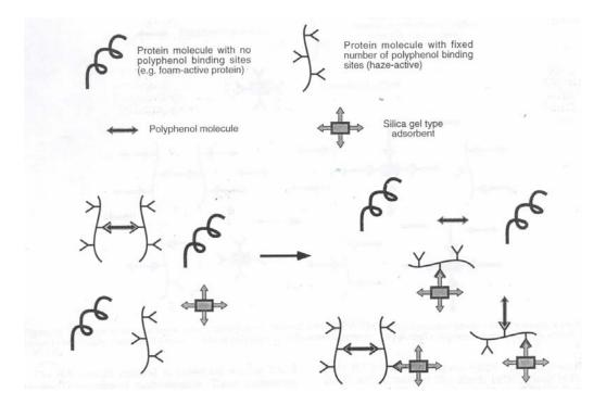
Figure 8. Mechanism of silica adsorption in high protein/polyphenol situation in beer. From "Mechanisms of Adsorbent action in Beverage Stabilization," K. Siebert & P. Lynn, 19997b, *Journal of Agriculture and Food Chemistry*. 45, 4275-4280.
