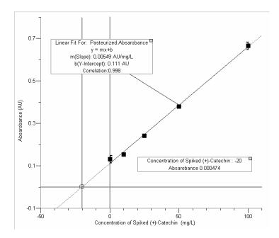
Figure D4. Concentration of (+)-catechin in pasteurized beer filtered with 20 lbs SHG/100 bbls
