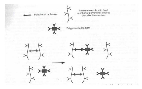
Figure 7. PVPP adsorption of beer haze-active polyphenols: PVPP is specific for haze-active polyphenols.
