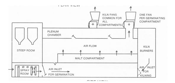
Figure 1. Diagram of typical malthouse.
