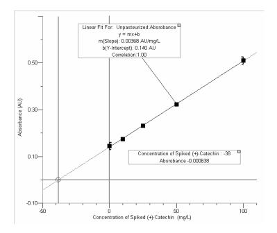
Figure D1. Concentration of (+)-catechin in unpasteurized beer coarse filtered.
