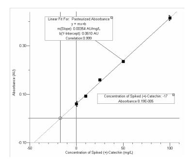
Figure D12. Concentration of (+)-catechin in pasteurized beer filtered with 10 lbs SHG/100 bbls and 8 lbs PVPP/100 bbls.
