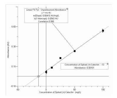
Figure D11. Concentration of (+)-catechin in unpasteurized beer filtered with 10 lbs SHG/100 bbls and 8 lbs PVPP/100 bbls.
