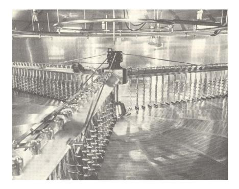
Figure 2. Interior of the lauter tun showing the lauter machine.
