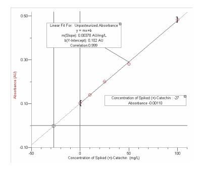
Figure D5. Concentration of (+)-catechin in unpasteurized beer filtered with 15 lbs SHG/100 bbls and 3 lbs PVPP/100 bbls
