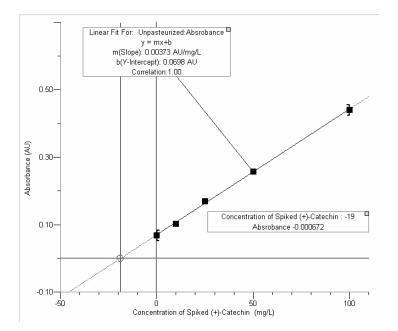
Figure D9. Concentration of (+)-catechin in unpasteurized beer filtered with 10 lbs SHG/100 bbls and 5 lbs PVPP/100 bbls.
