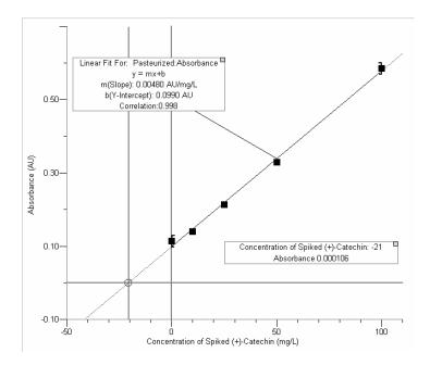
Figure D2. Concentration of (+)-catechin in pasteurized beer coarse filtered.
