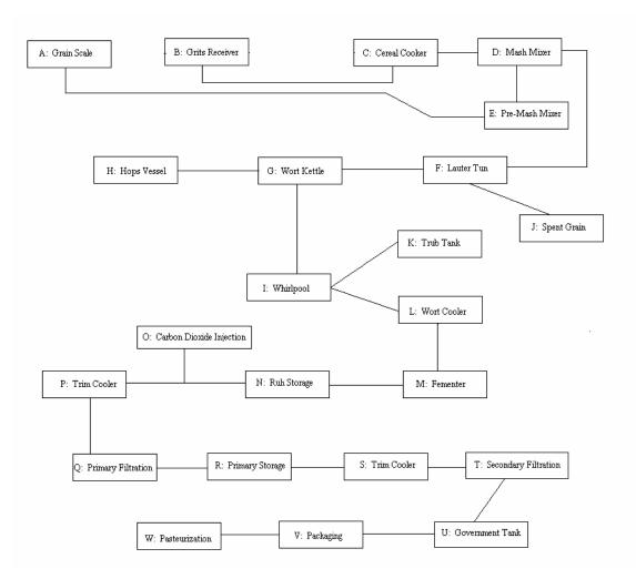
Figure 11. Flow chart of raw materials through the plant in beer processing
