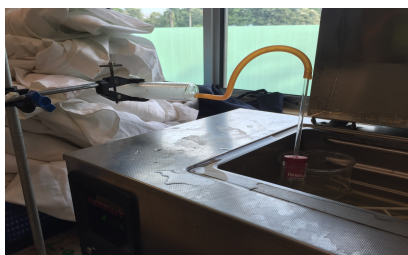
A photograph taken by myself using an iPhone 6, on 26/04/2016, that displays the experiment in progress in the Memmert water bath, with the mixture of catalase (0.1%) and \text{H}_2\text{O}_2 ( 0.01\text{ moldm}^{-3} ) in the test tube, connected to a glass gas syringe held by a retort stand
