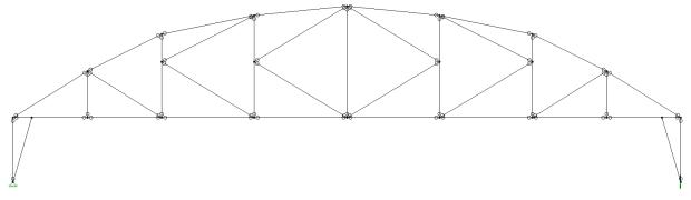
Figure 2-2: Parker (K) Truss Alternative Elevation View
