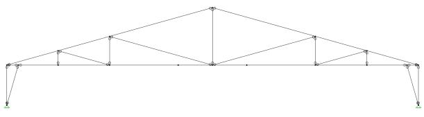
Figure 2-1: Double Howe (KK) Truss Alternative Elevation View
