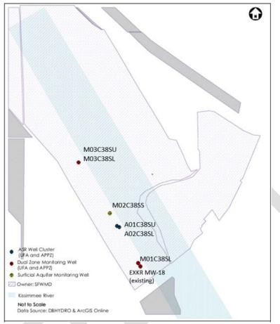
Figure 3-1. C-38S ASR test well and monitoring well layout.
