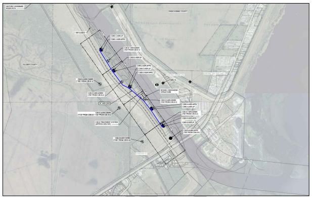
Figure 5-1. Conceptual layout of the C-38S ASR wellfield.
