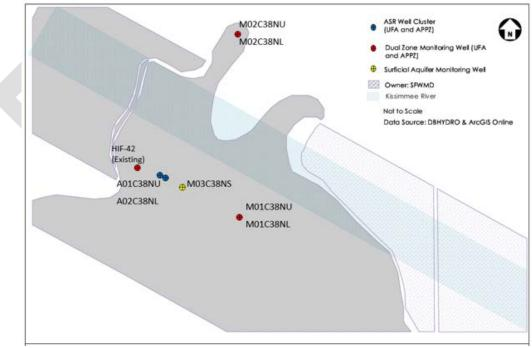
Figure 3-2. C-38N ASR test well and monitoring well layout.
