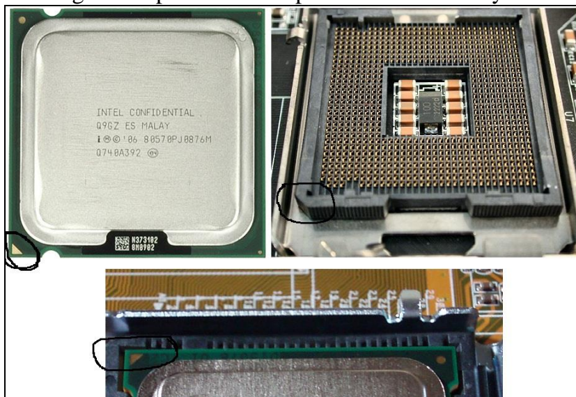
Figure 3.5 Processor and Processor Socket direction for assembling
