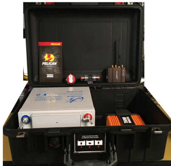
Figure 4 - Generation 1 of Power Pack (Battery, Inverter, Mobile Modem)
