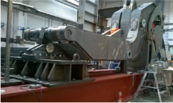
Figure 8. Fatigue test of the boom structure in laboratory of Steel Structures at LUT and simulation model for the same structure
