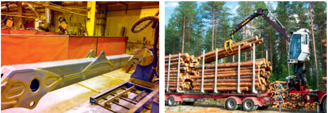
Figure 2. Novel Kesla UHSS truck crane boom (left) and the final product in operation (right)
