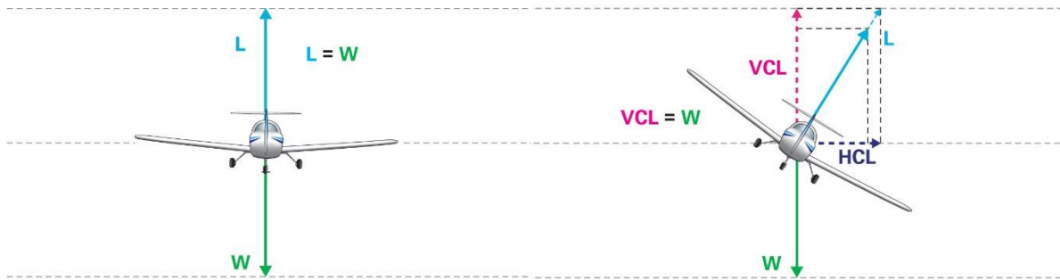
Figure 2 Forces in level flight and in the 45° angle of bank turn
