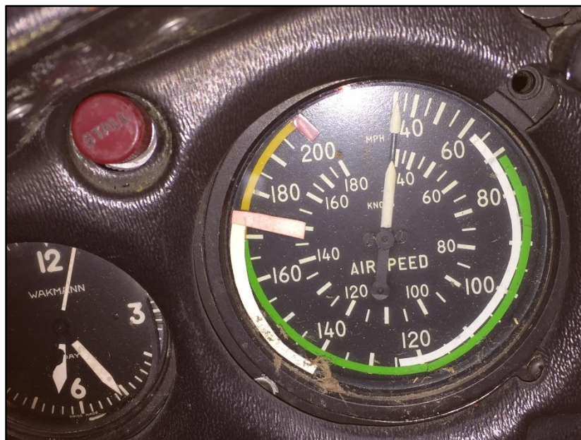
Figure 7 Airspeed indicator and stall warning light (upper left)
