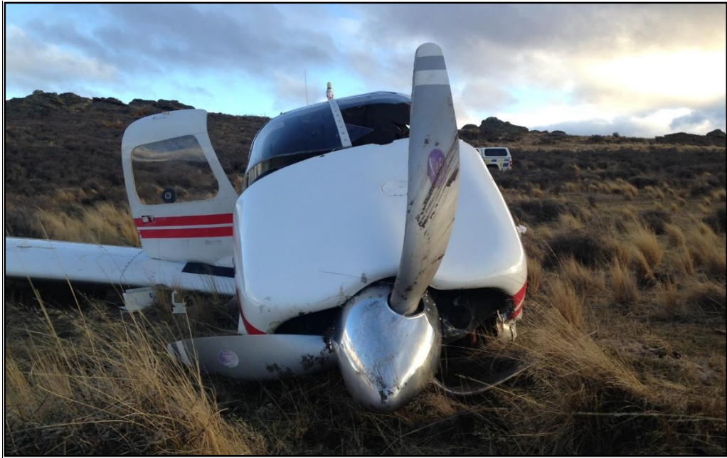
Figure 4 Damage to propeller
