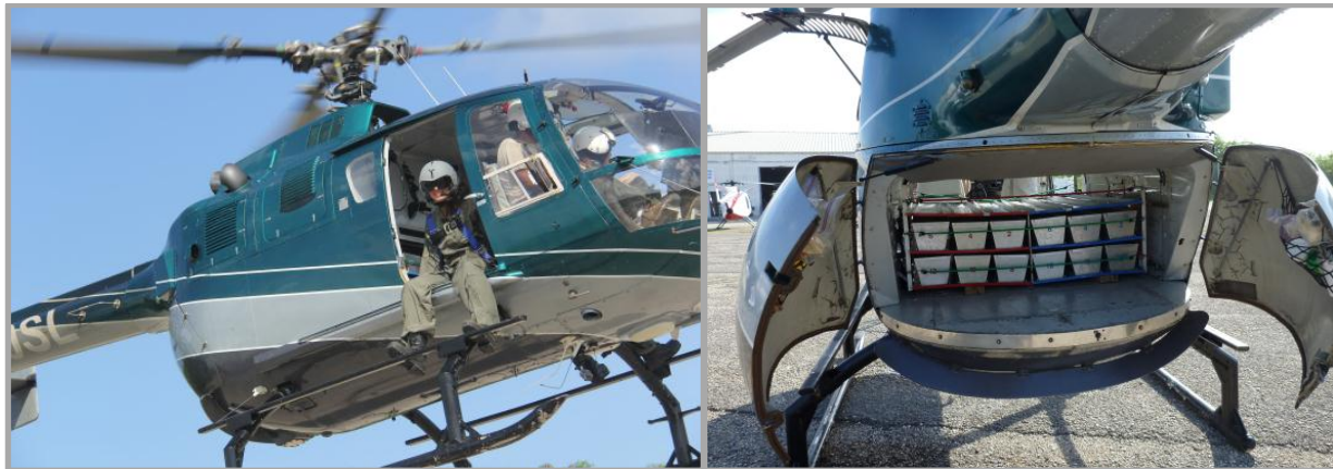
Figure 19. Bolkow 105 Helicopter and crew in preparation for aerial deployment of DNM treated with an 80 mg acetaminophen tablet to control brown tree snakes. Racks in image to the right contain DNM baits attached to flaggers.
