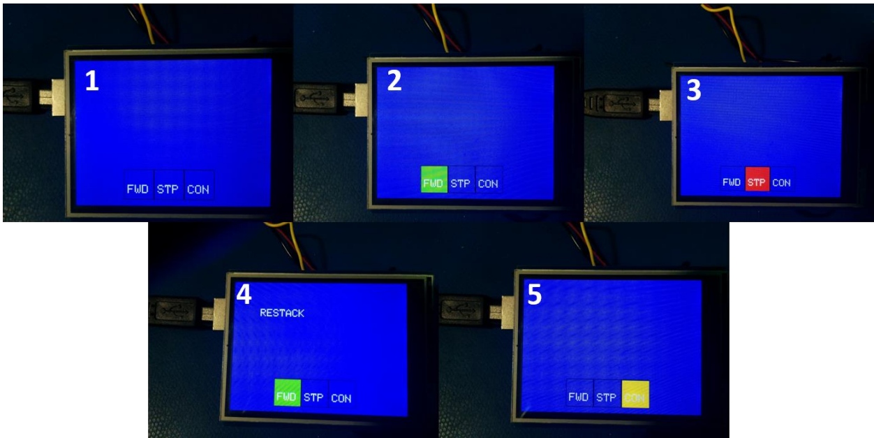
Figure 20: Different displays of the off-board controller depending upon the commands pressed on the touchscreen LCD device by the user. The respective command is sent to the robot's on-board controller via serial communication for its operation.
