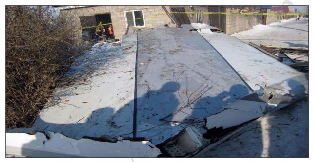
Figure 29. RH wing tip with winglet
