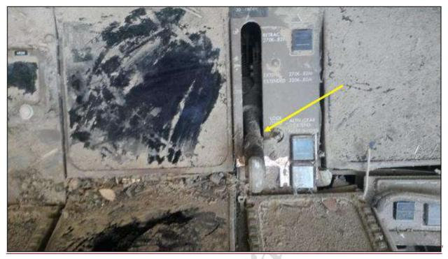
Figure 7. Landing gear extension/retraction control lever
