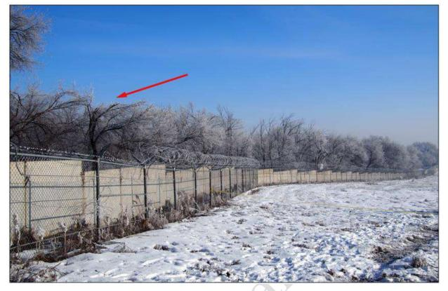
Figure 26. Trees damaged by aircraft RH wing tip (indicated by arrow) The aircraft first touchdown occurred at the distance of  $\approx$ 900 m from the end of RWY at the cross track angle of  $\approx$ 40 m to the right from the continued RWY coordinated axis.
