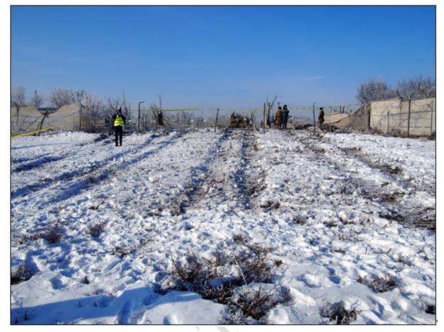
Figure 27. Main landing gear wheel traces at first touchdown place
