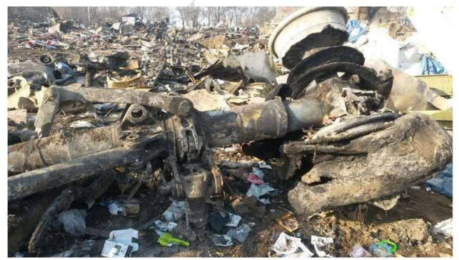
Figure 6. Nose landing gear
