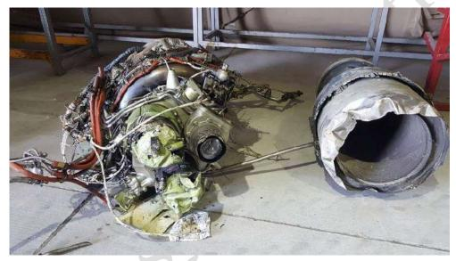
Figure 17. Dismantled APU with APU exhaust nozzle
