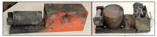
Figure 12. Inboard flight data monitoring and recording equipment
