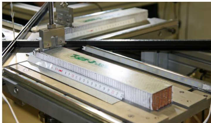
Figure 12. Clamping of the specimen to the test fixture
