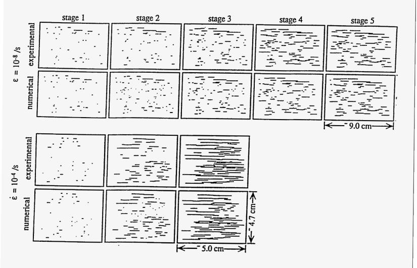
Figure 3: Comparison of experimental and numerical fracture sets. Fracture sets were experimentally generated at the strain rates indicated using brittle coating techniques (Wu and Pollard, 1991). Many of the small flaws in the numerical simulation do not show up in the experimental simulation because they have not grown long enough to be visible. The thickness of the brittle coating is ~0.02 cm (Renshaw and Pollard, 1991).
