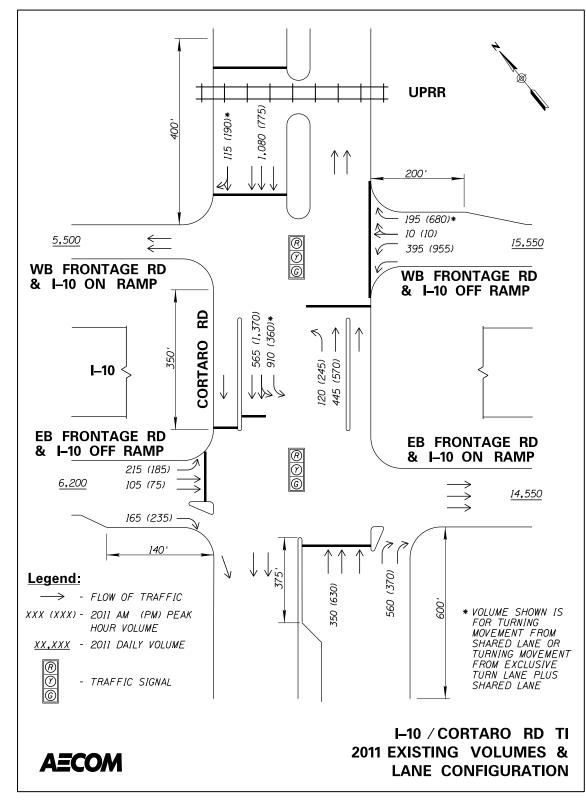
Figure 2.12 – I-10/Cortaro Road TI 2011 Existing Volumes & Lane Configuration
