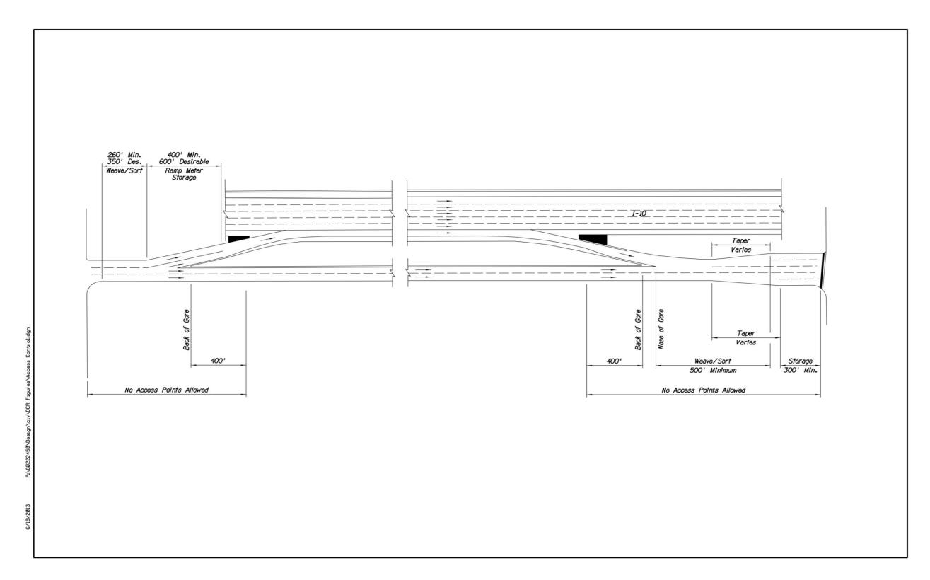
Figure 4.1 – Access Control at Ramp/Frontage Road with Crossroad
