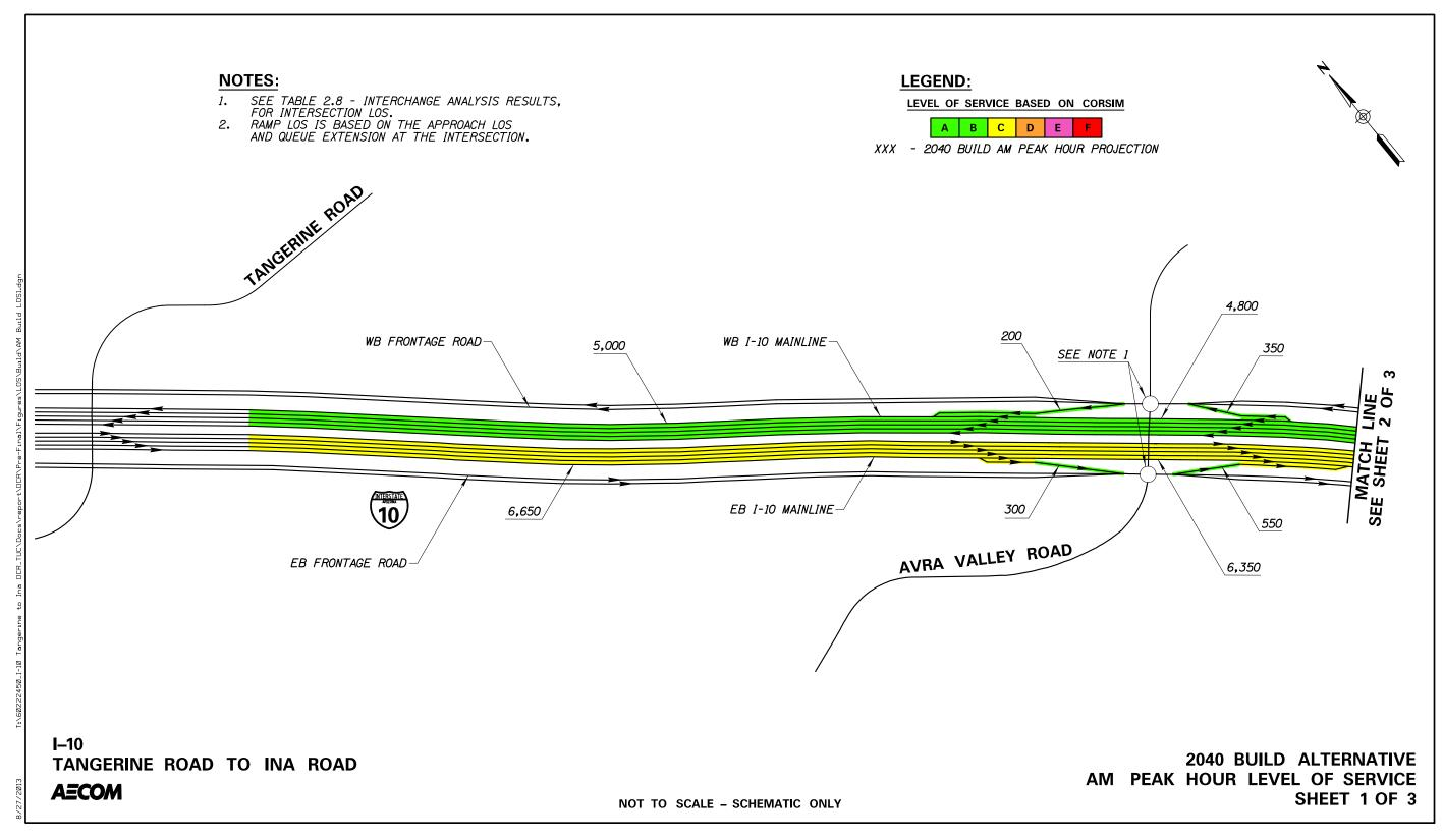
Figure 2.9 – 2040 Build Alternative AM Peak Hour Level Of Service
